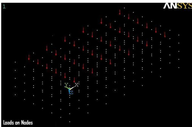
Fig. 5 Applied Loads at the Foundation Nodes
