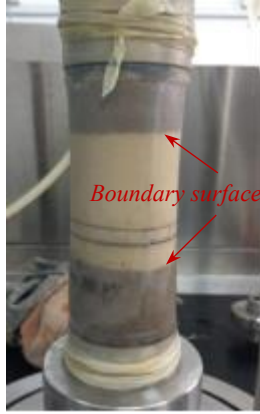
132 Fig. 4. The triaxial specimens preparation. (a) 60mm powdery interlayer; (b) 2×20mm powdery layers.
