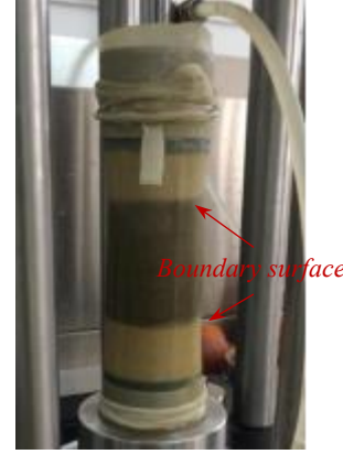
132 Fig. 4. The triaxial specimens preparation. (a) 60mm powdery interlayer; (b) 2×20mm powdery layers.
