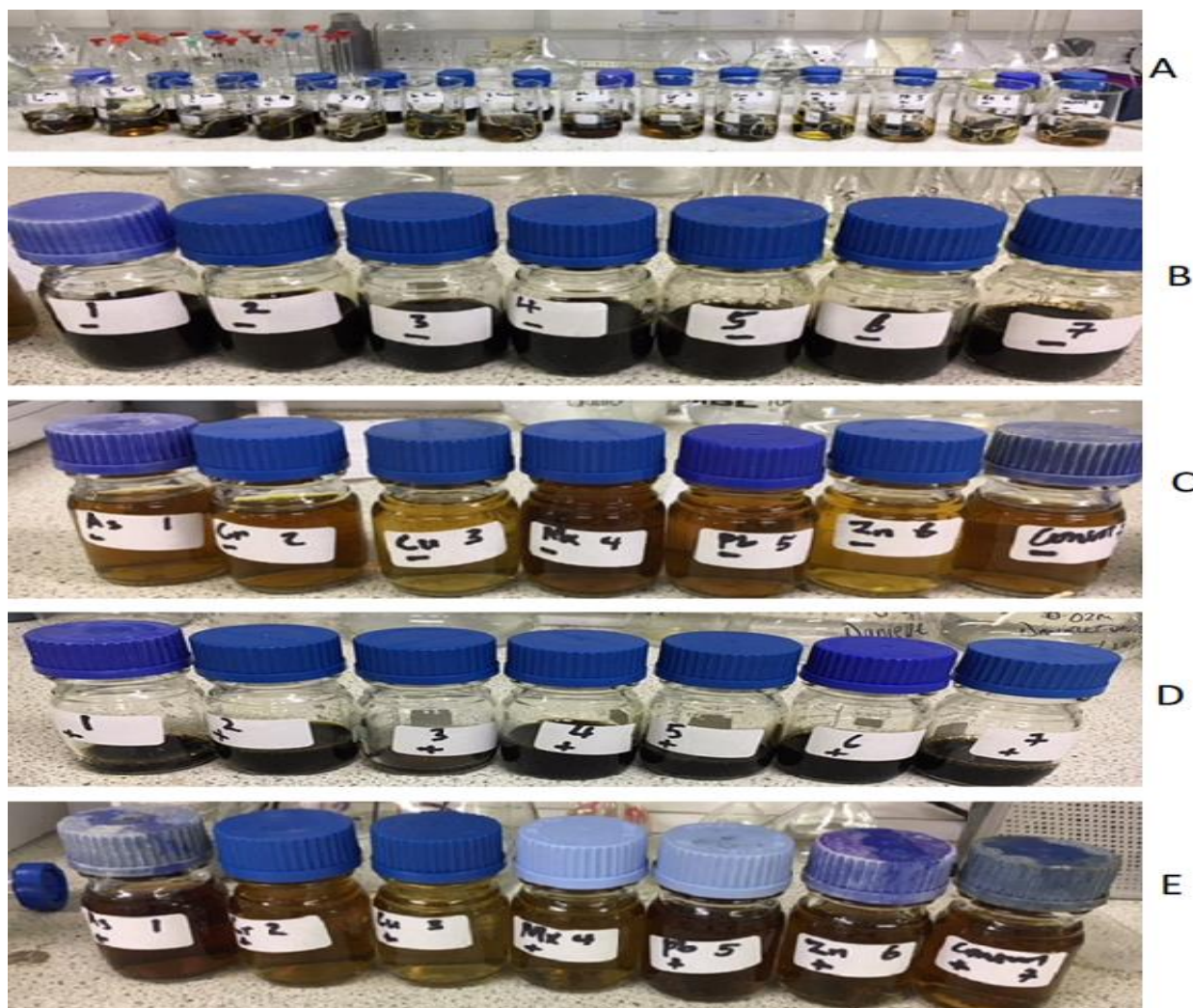
Figure 6. 2 Dialyzed humic and fulvic samples before freeze drying process (A= dialysis process, B and C= humic acid (HA) fractions before and after dialysis, respectively, D and E= fulvic acid (FA) fractions before and after dialysis, respectively)
