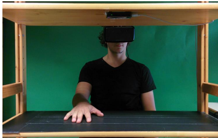
Figure 75. Example of experimental setup with Leap Motion fixed to shelf (taken from Argelaguet et al., 2016).
