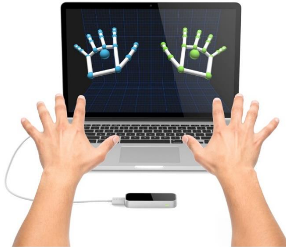
Figure 5. Leap Motion device and example basic virtual hands.
