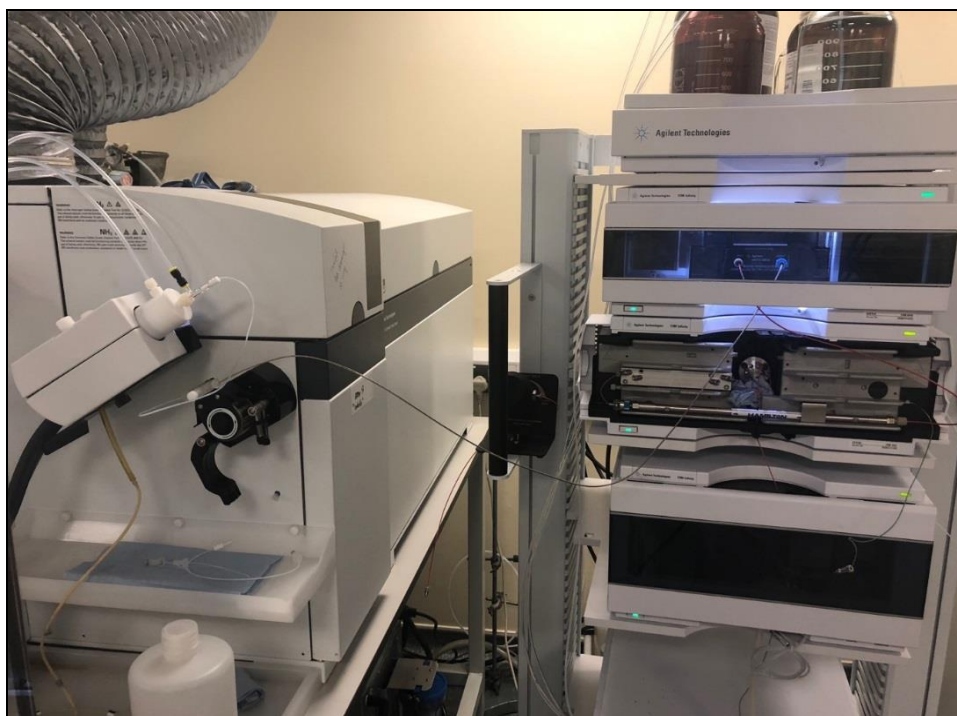
Figure 4.4 High-performance liquid chromatography-inductively coupled plasma mass spectrometer (HPLC-ICP-MS) used to analyse arsenic species in the shrimp
