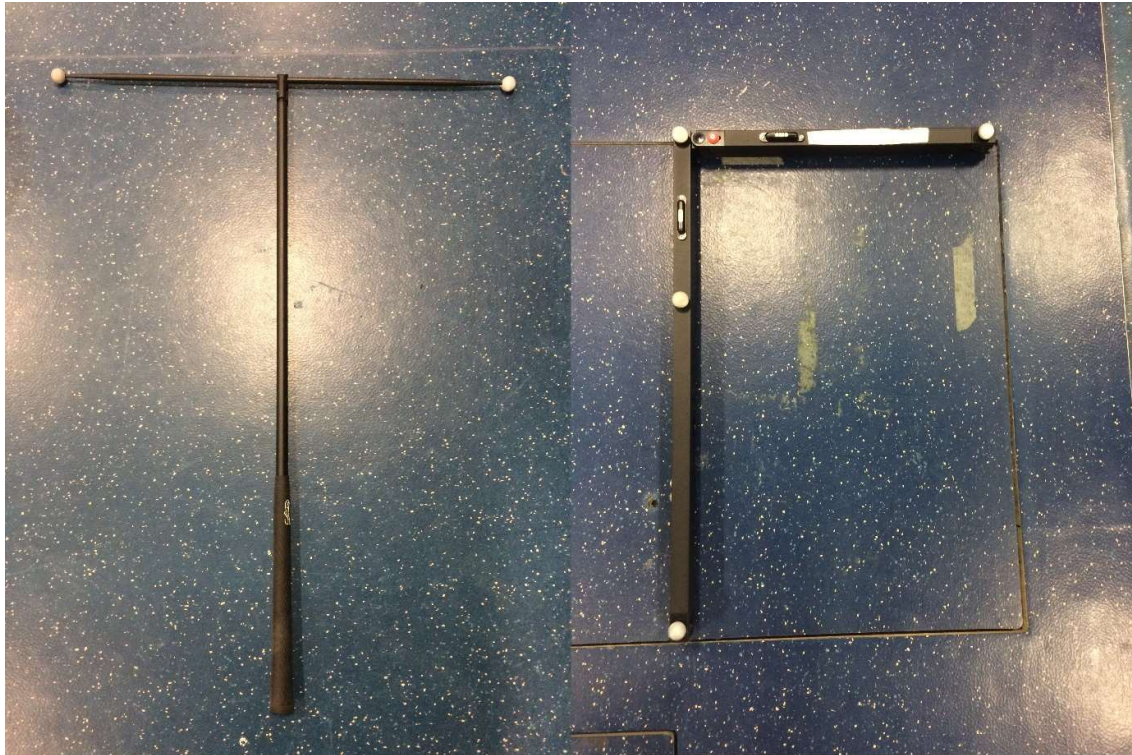
Figure 3-8 The wand equipped with two markers and the L-shaped metal frame.
