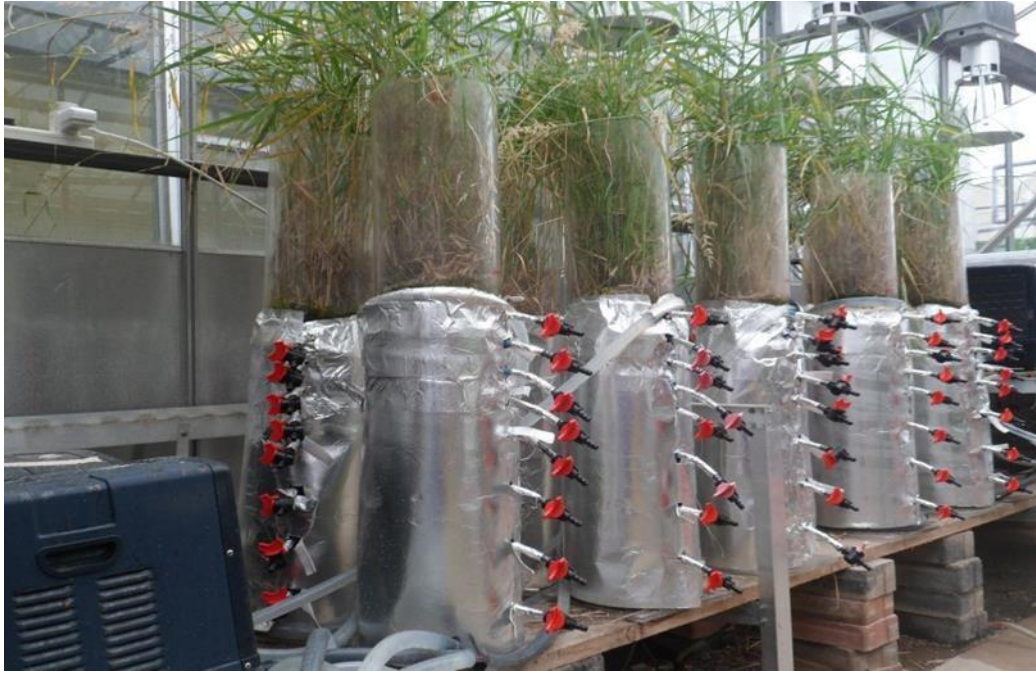
Figure 3.2: Laboratory Set-up of the Vertical-flow Constructed Wetland Note: that the above set up includes two filters in the middle (filter 5 and 6) that are not in operation. They serve as controls receiving clean de-chlorinated water.
