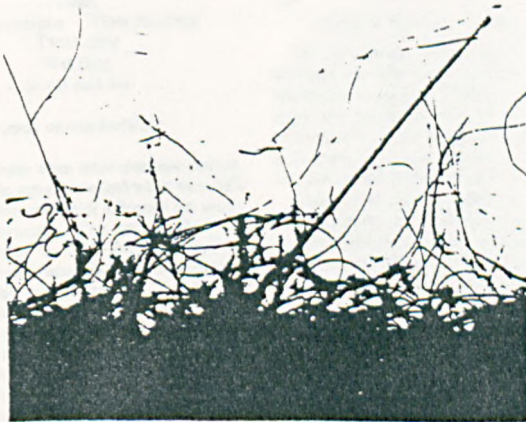
A fabric surface profile showing surface hairiness. This fabric caused discomfort due to tickle and fibre shedding (X 8).
