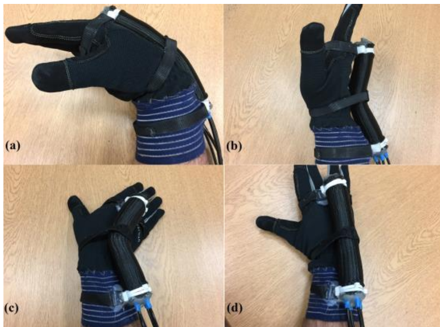
Figure 7.37: Wrist rehabilitation exercises based on the new version of the wrist rehabilitation prototype.
