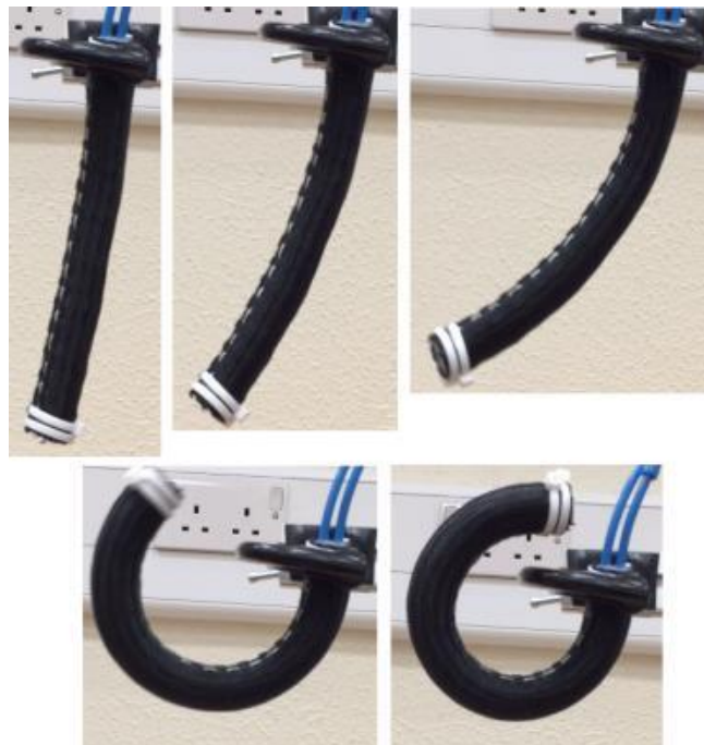
Figure 7.5: The novel controllable stiffness bending actuator.
