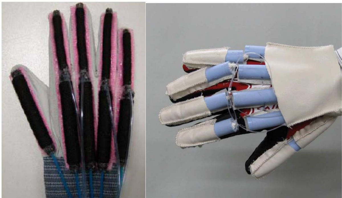
Figure 2.9: (a) Two Joints Power Assisted Glove (Noritsugu et al., 2008); (b) Power-Assist Glove (Toya, Miyagawa, & Kubota, 2011).
