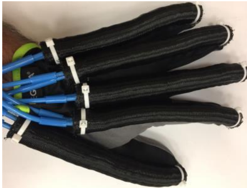
Figure 7.6: Rehabilitation glove based on controllable stiffness bending muscles.
