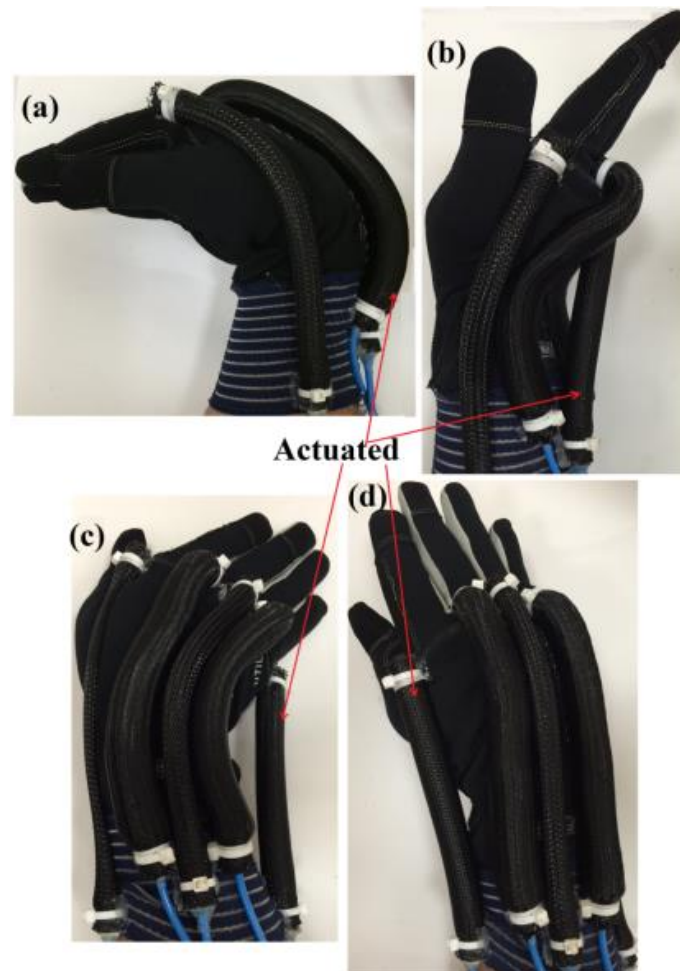
Figure 7.34: The rehabilitation movements of the proposed wrist soft exoskeleton: (a) Wrist flexion movement, (b) Wrist extension movement, (c) Wrist ulnar deviation movement (d) Wrist radial deviation movement.
