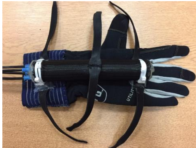
Figure 7.36: Wrist rehabilitation exoskeleton based on ABPAM.
