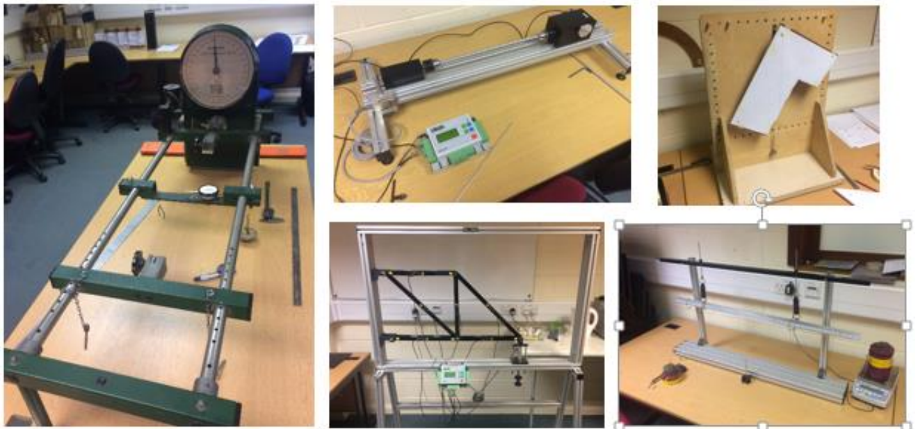
Figure 7.1.1 Structural laboratory apparatus at the University of Salford. From Left to right, Buckling of struts, Torsion of circular shafts, Pin-jointed frameworks, Centroids of area, Beam reactions & static equilibrium
