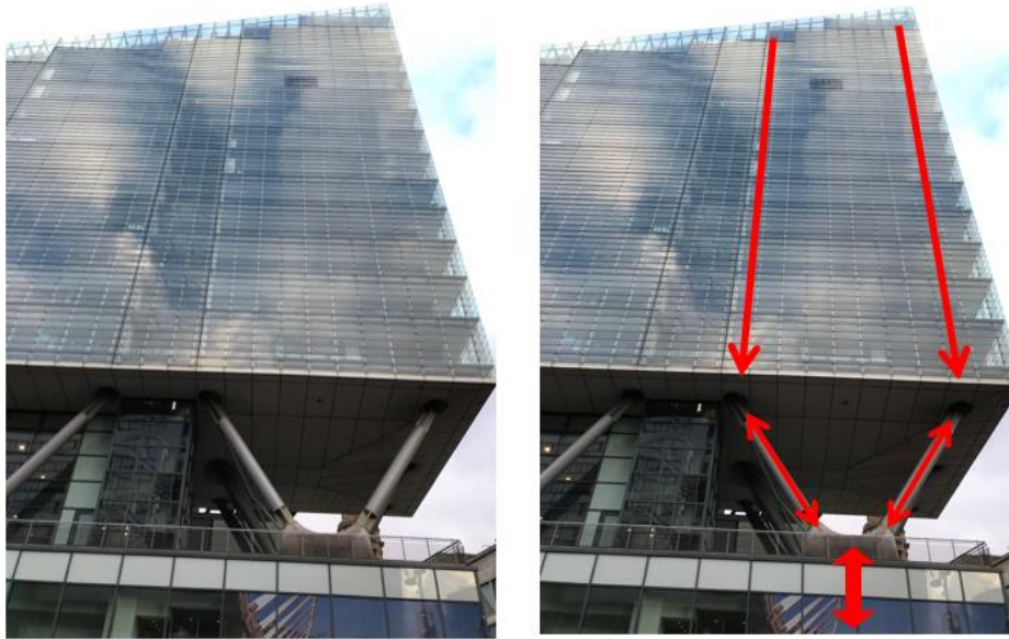
Figure 6.1.9 Animations show how the structural load paths down through the structure using animated arrows.
