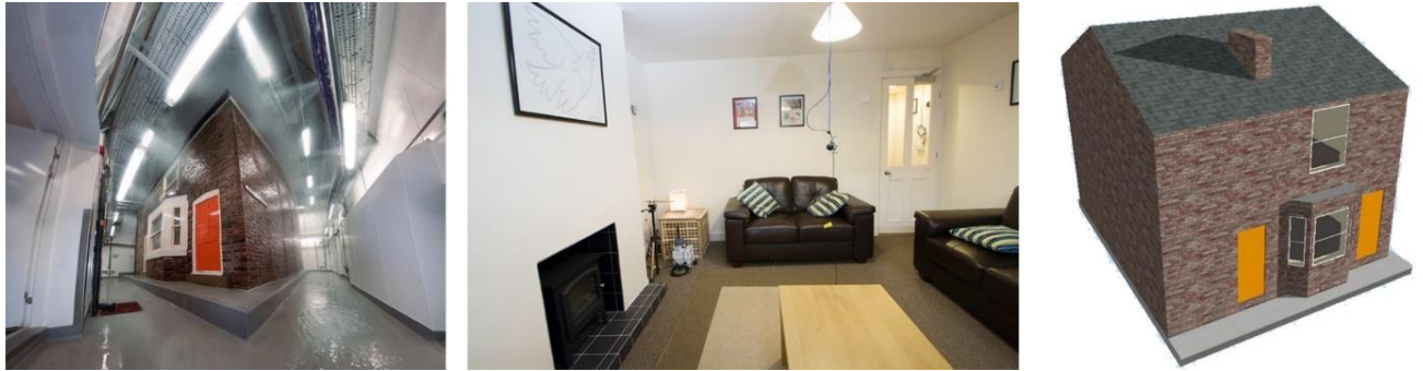
Figure 4: Left: The Energy House within the climate controlled chamber at the University of Salford. Middle: A view from the living room of the House. Right: The corresponding DesignBuilder model of the House.
