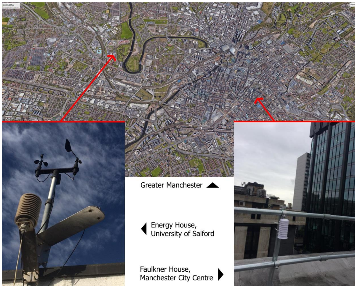
Figure 1: Top: The aerial view of Manchester (image from Google Maps). Left: The weather station on the roof of the Energy House building at the campus of the University of Salford. Right: HOBO data logger installed on the roof of the Faulkner House in Manchester city centre.
