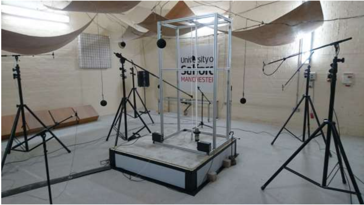
Figure 7: Drop test assembly on the bare concrete floor in the reverberation chamber.
