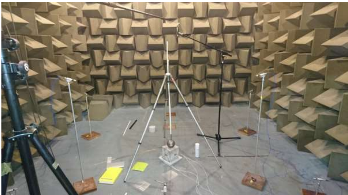
Figure 3: Experimental test setup employed in the semi-anechoic chamber.
