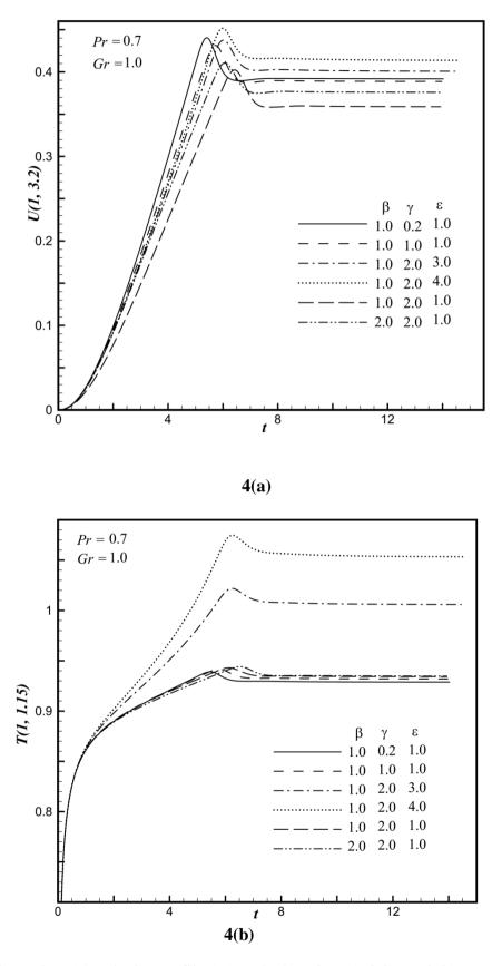
**Fig. 4.** Time-dependent (a) velocity profile (*U*) at the location (1, 3.2); and (b) temperature profile (*T*) at the location (1,1.15) versus time (*t*) for various values of  $\beta$ ,  $\gamma$  and  $\varepsilon$ .
