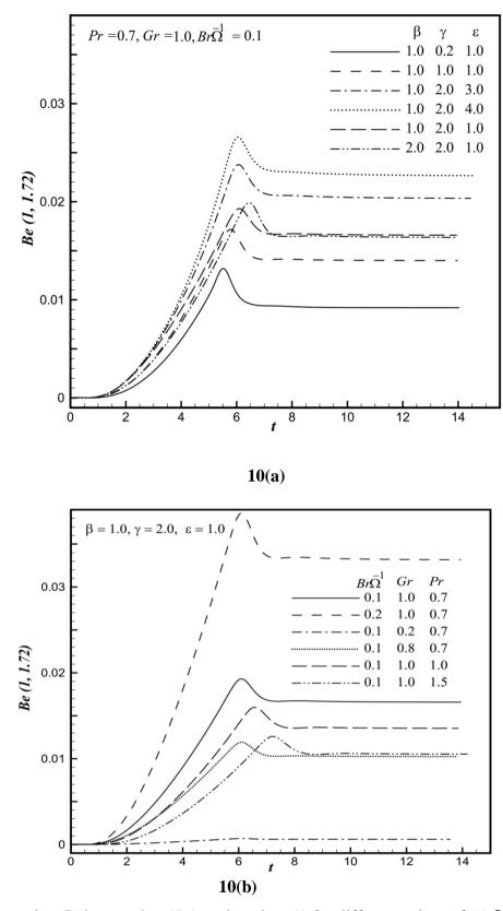
**Fig. 10.** The transient Bejan number (*Be*) against time (*t*) for different values of (a)  $\beta$ ,  $\gamma$  and  $\epsilon$ ; & (b)  $Br\Omega^{-1}$ , Gr and Pr.
