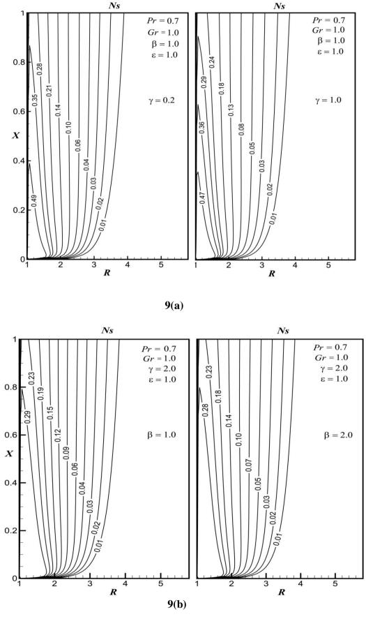
**Fig. 9**. The steady-state entropy contours (*Ns*) for different values of (a)  $\gamma$ ; and (b)  $\beta$ .
