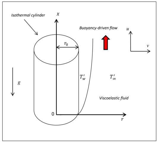
Fig. 1. Physical model of the analysis.
