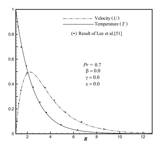
Fig. 2. Comparison of the flow-field variables with existing available results Lee et al. [51].
