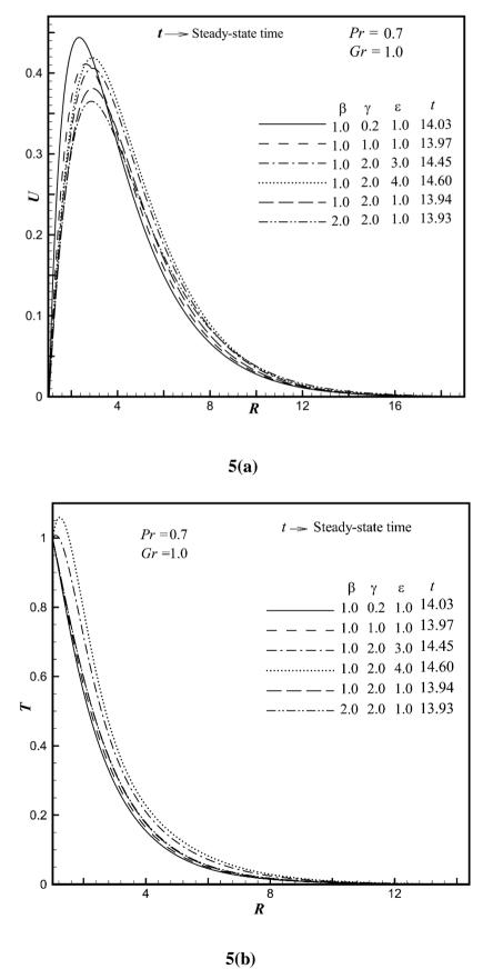
**Fig. 5**. Simulated time-independent state (a) velocity (*U*); and (b) temperature (*T*) profiles versus *R* at X = 1.0 for various values of  $\beta$ ,  $\gamma$  and  $\varepsilon$ .
