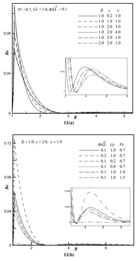
**Fig. 11.** The steady-state entropy Bejan number (*Be*) versus R at X = 1.0 for various values of (a)  $\beta$ ,  $\gamma$  and  $\varepsilon$ ; & (b)  $Br\Omega^{-1}$ , Gr and Pr.
