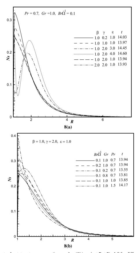
**Fig. 8.** The steady-state entropy generation number (*Ns*) against *R* at X = 1.0 for different values of (a)  $\beta$ ,  $\gamma$  and  $\varepsilon$ ; & (b)  $Br\Omega^{-1}$ , Gr and Pr.
