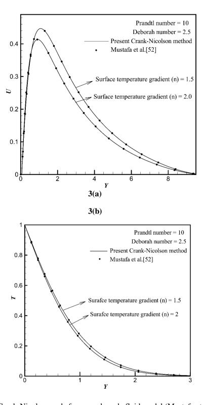
**Fig 3.** Validation of Crank-Nicolson code for second-grade fluid model (Mustafa et al. [52]) with respect to (a) velocity profile; (b) temperature profile.
