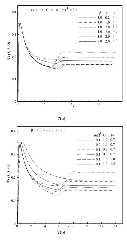
**Fig. 7.** The transient entropy generation number (*Ns*) against time (*t*) for different values of (a)  $\beta$ ,  $\gamma$  and  $\varepsilon$ ; & (b)  $Br\Omega^{-1}$ , Gr and Pr.
