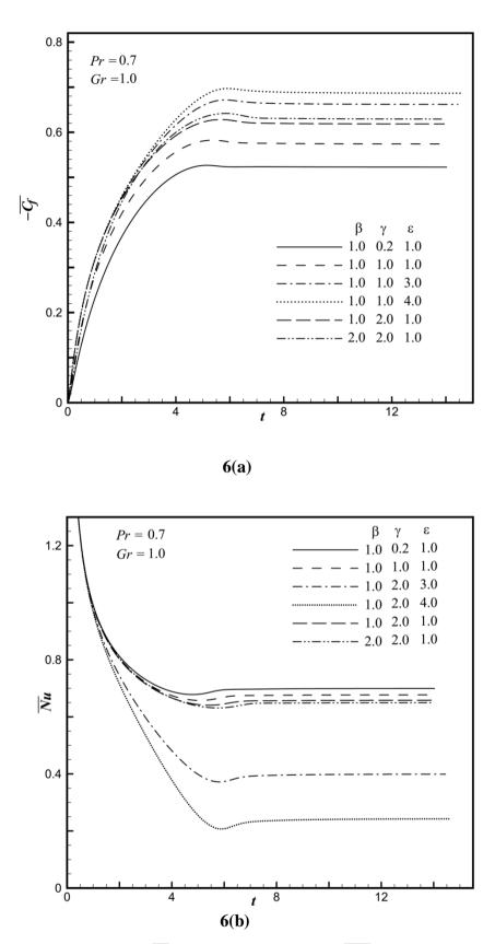
**Fig. 6.** Average (a) skin-friction  $(\overline{C_f})$ ; and (b) heat transport  $(\overline{Nu})$  coefficients for distinct values of β, γ and ε.
