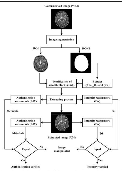
**Fig. 4** Process diagram for the extraction and verification process. Starts by segmenting the watermarked image into ROI and RON. Smooth blocks inside ROI are then identified. Watermark is extracted from the identified smooth blocks. The watermark is compared to the recalculated watermark of the extracted image to verify the authenticity and integrity of the image
