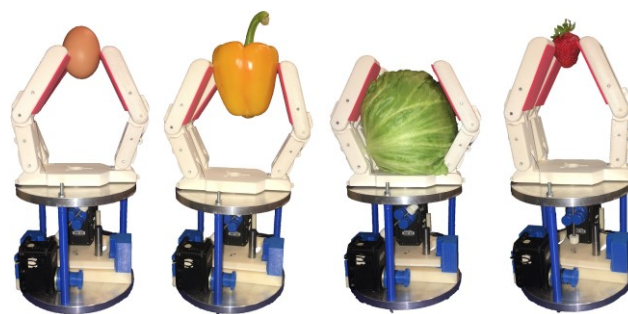
FIGURE 10. VSH 1 with three finger can grasp different objects with different sizes and flexibilities thanks to its variable stiffness mechanism.
