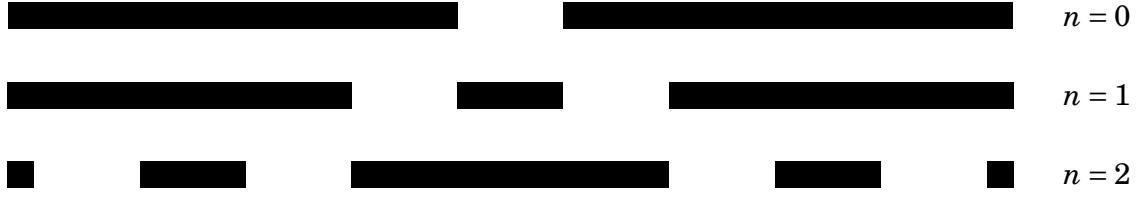
Figure 3.8: A modified Cantor grating with a static a_n value. One can see how quickly the overall grating size grows as n increases.
