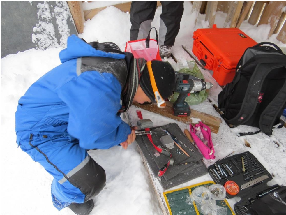
Figure 4-13: Making holds on collar before fitting dosimeter box
