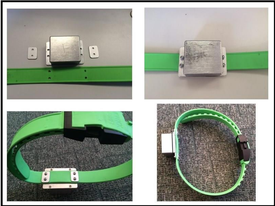
Figure 4-4: Testing mounting of the dosimeter box on a large mammal GPS collar
