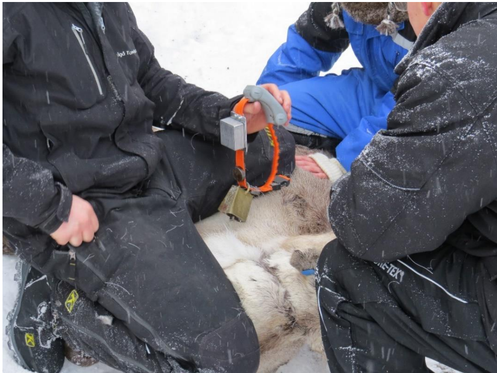
Figure 4-14: Dosimeter box mounted on the collar preparing to reattach to a reindeer
