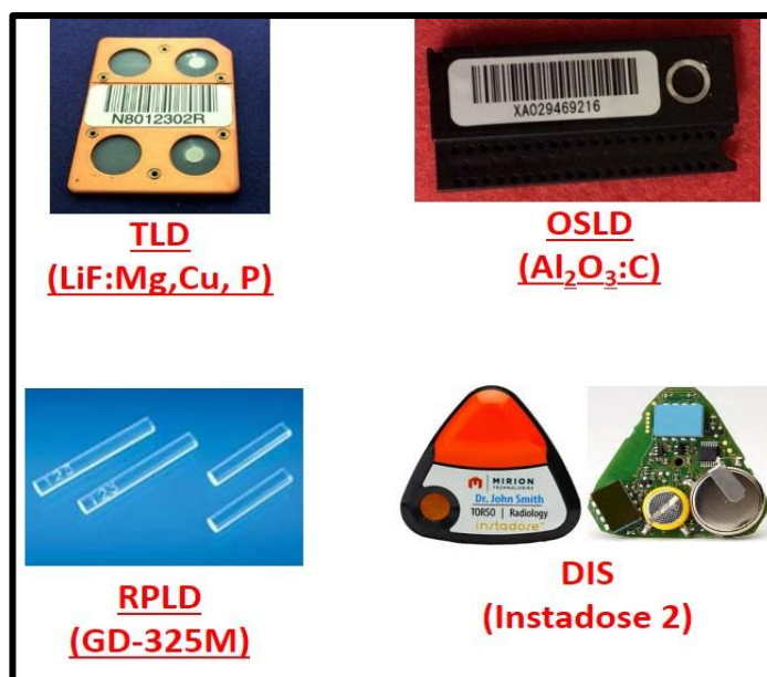
Figure 4-2: Dosimetry technologies used for measuring external doses of large mammals
