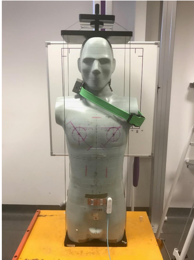
Figure 4-17: Applied deer phantom loaded TLDs in and attached dosimeter box at the neck of the phantom for irradiated to x-ray (50 kVp (100 mAs) and 100 kVp (100 mAs)) and gamma radiation ( ^{137}\text{Cs} , 662 keV)
