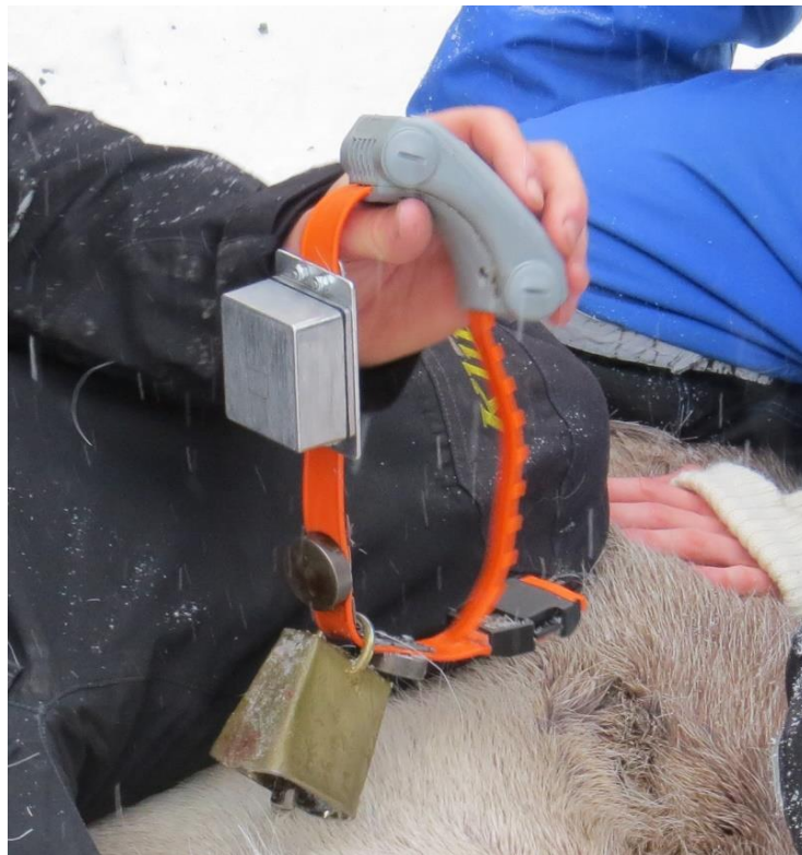
Figure 6-2: A dosimeter box attached onto a reindeer GPS collar and counterweights
