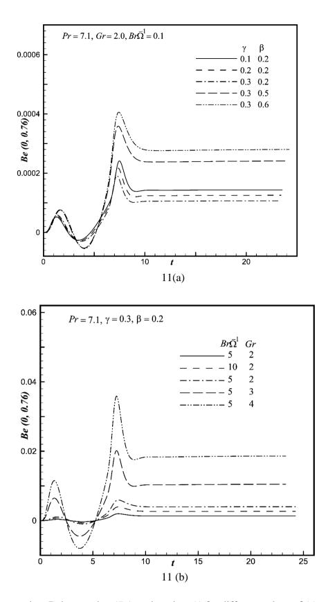
Fig. 11. The transient Bejan number (*Be*) against time (*t*) for different values of (a)  $\gamma$  and  $\beta$ ; & (b)  $Br\Omega^{-1}$  and *Gr*.
