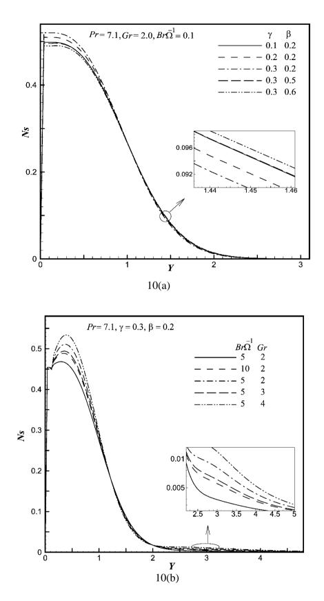
Fig. 10. The steady-state entropy generation number (*Ns*) against *Y* at *X* = 1.0 for different values of (a)  $\gamma$  and  $\beta$ ; & (b)  $Br\Omega^{-1}$  and *Gr*.
