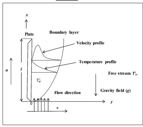
Fig. 1: Flow geometry and coordinate system.
