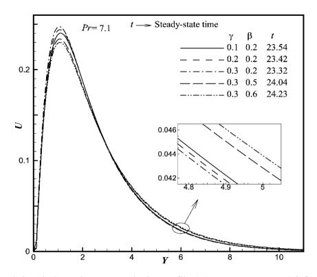
Fig. 4. Simulated time-independent state velocity profile (*U*) versus *Y* at *X* = 1.0 for various values of  $\gamma$  and  $\beta$ .
