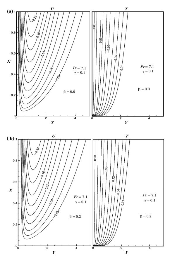
Fig. 15. The steady-state velocity (*U*) and temperature (*T*) contours for (a) Newtonian fluid ( $\beta = 0.0$ ); and (b) second-grade fluid ( $\beta = 0.2$ ).
