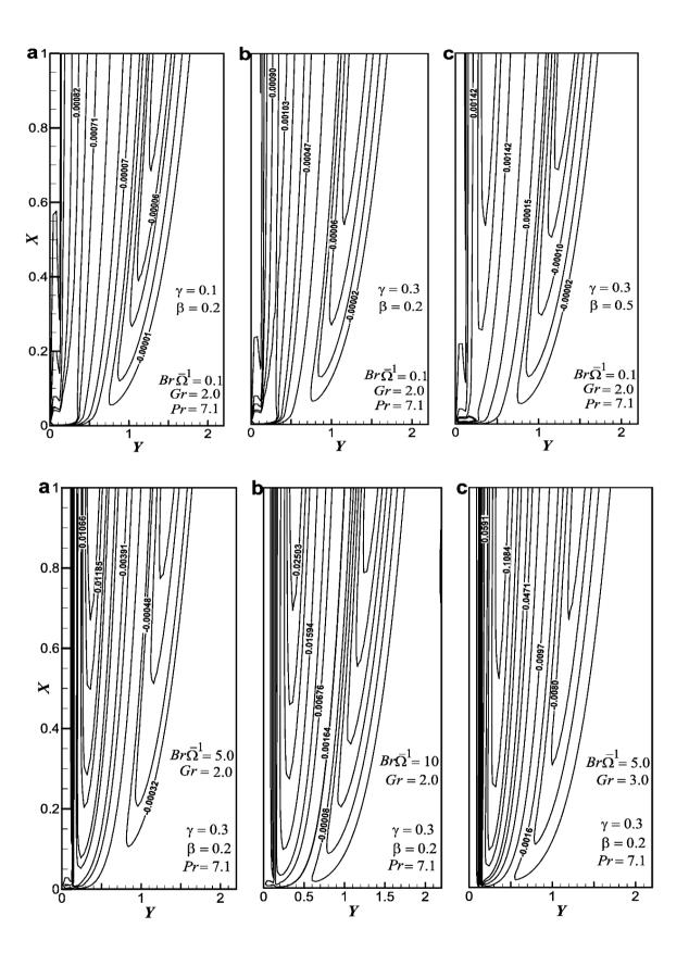
Fig. 14a,b. The steady-state Bejan contours (*Be*) for different values of (a)  $\gamma$  and  $\beta$ ; & (b)  $Br\Omega^{-1}$  and *Gr*.
