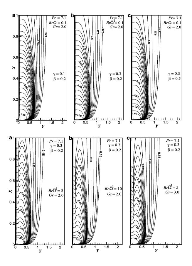
Fig. 13a,b. The steady-state entropy contours (*Ns*) for different values of (a)  $\gamma$  and  $\beta$ ; & (b)  $Br\Omega^{-1}$  and *Gr*.
