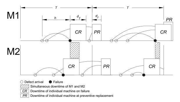
Figure 1. Two machines (M1 and M2) in parallel, subject to defect arrivals  $\circ$ , failures  $\bullet$ , periodic inspection interval T, downtime  $d_f$  due to corrective replacement, CR, on failure, and downtime  $d_r$  ( $d_r < d_f$ ) due to preventive replacement, PR, on defect found at inspection.
