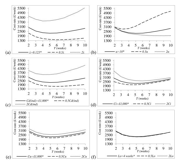
Figure 7. Sensitivity of the cost-optimal policy (\*baseline) to: (a) defect arrival rate; (b) failure *delay-time*; (c) individual machine downtime cost-rate; (d) inspection cost; (e) unit cost; and (f) lead-time.
