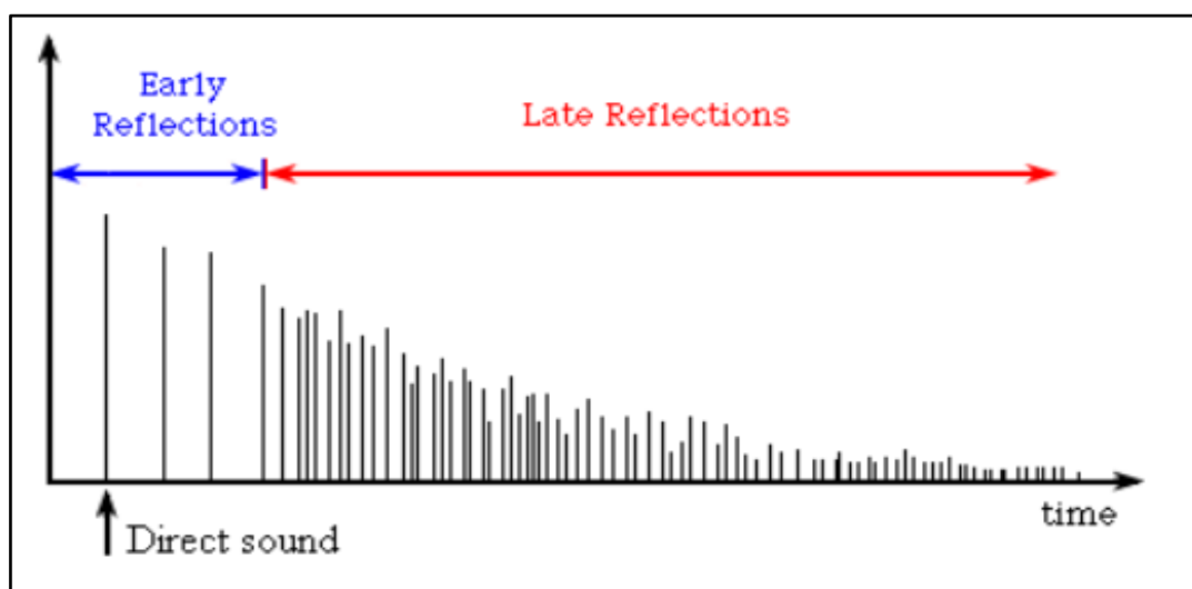
Figure 2.10 the main parts of impulse response
