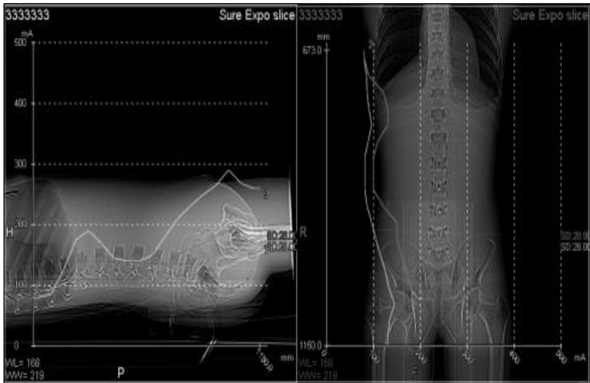
Figure 2- 18: Schematic diagram illustrating the AP and lateral scout views which in combination with SD values aid the determination of tube current values for CT scans of the abdomen. (Nivelstein, Van Dam, & Van Der Molen, 2010)
