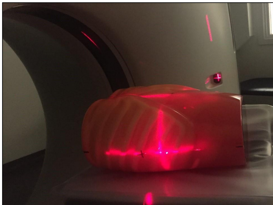
Figure 5- 8: Anthropomorphic abdomen phantom position, the CT laser lights were used as a positioning aid.
