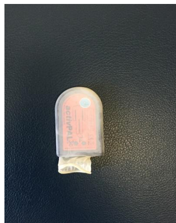
Figure 8 activPAL™ in waterproof dressing
