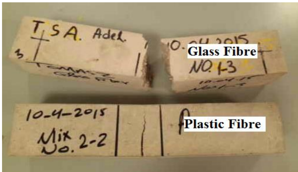
Figure 4.32: Comparison between the effect of Glass fibre and Plastic fibre reinforcement on crack type
