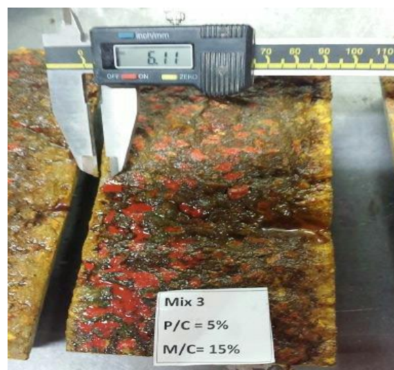
Figure 5.22: Measuring depth of chloride ion penetration for modified concrete
