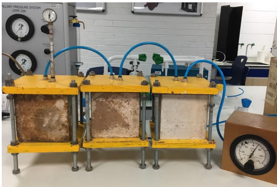
Figure 3.17: Gas penetration (carbonation) under pressure test device.
