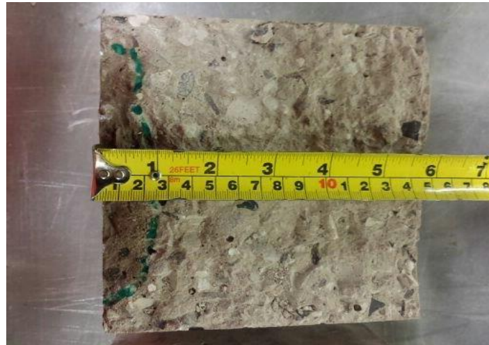
Figure 5.27: Section of modified concrete specimen shows depth of water penetration under 5 bar pressure
