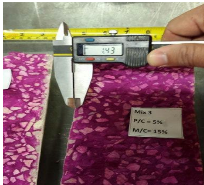
Figure 5.19: Measuring depth of carbonation of modified concrete by 15% partial replacement of metakaolin and 5% polymer
