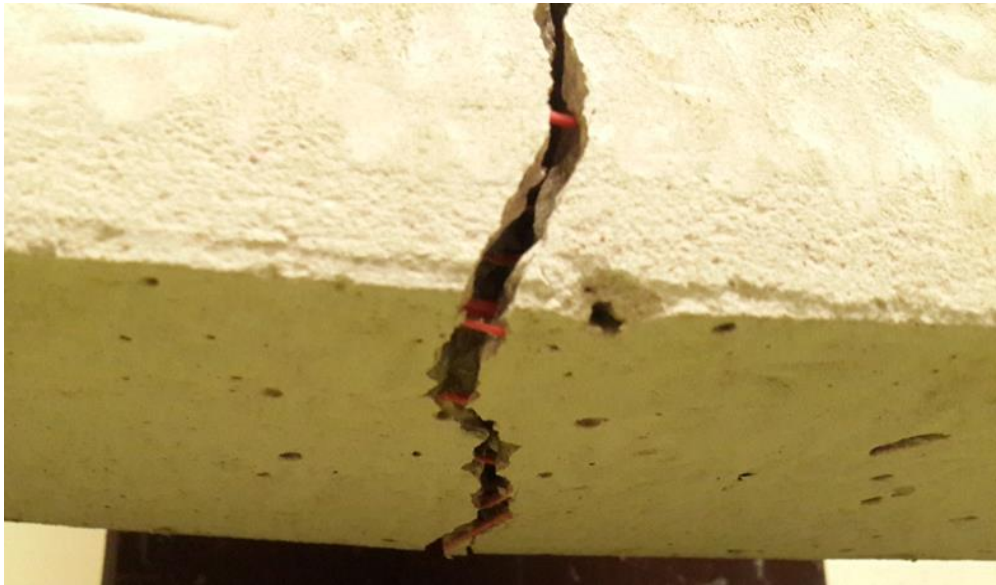
Figure 4.31: Effect of plastic fibre reinforcement on crack zone
