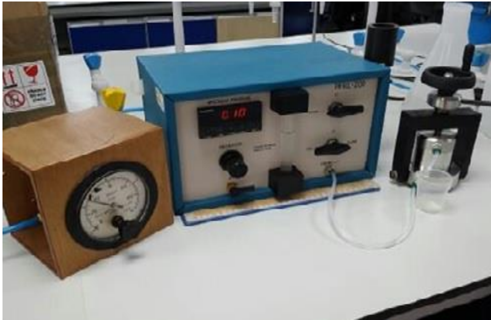
Figure 3.14: PERL-200 device to measure water permeability for concrete and mortar
