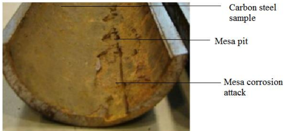
Figure 2-9: Mesa corrosion attack on carbon steel [25]
