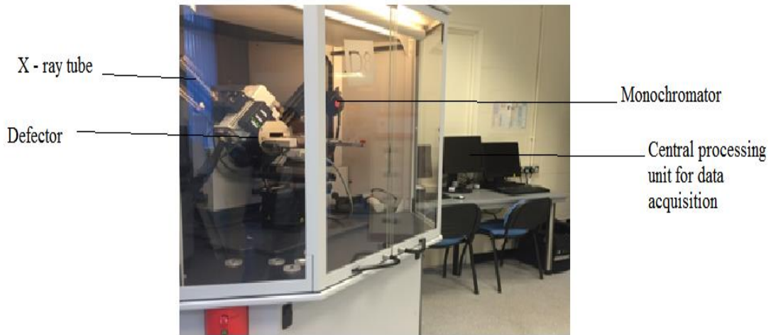
Figure 3-15: A typical image of XRD for specimen's surface analysis
