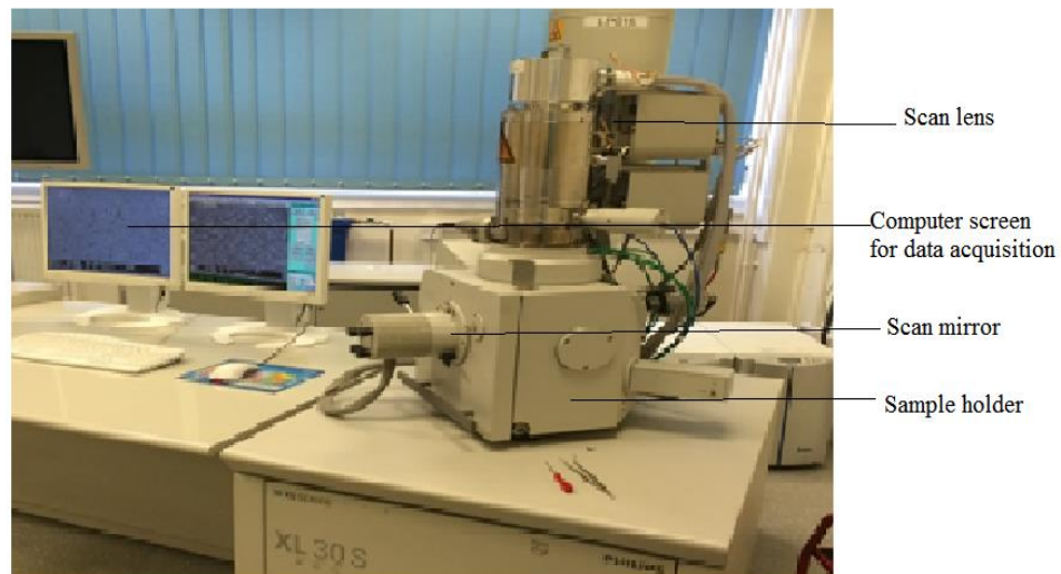
Figure 3-14: A typical image of SEM for specimen's surface analysis.
