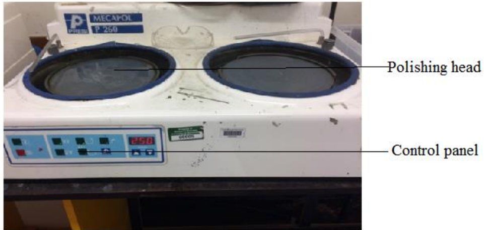
Figure 3-6: Mechanical polishing machine in preparation for tests
