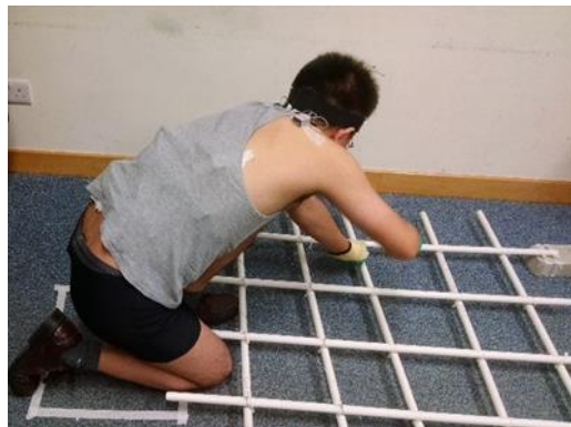
Figure 2: Laboratory rebar tying setup
