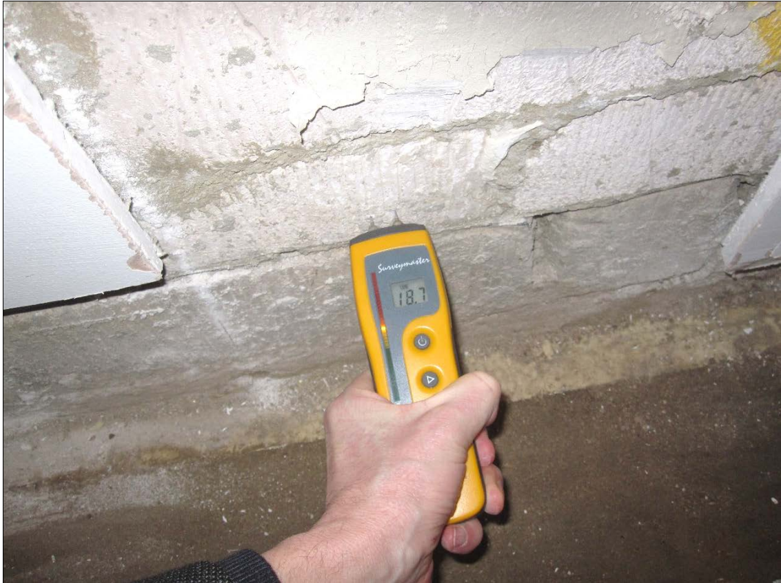
Figure 41: Protimeter Surveymaster meter: measure-mode function using the integrated pins.
