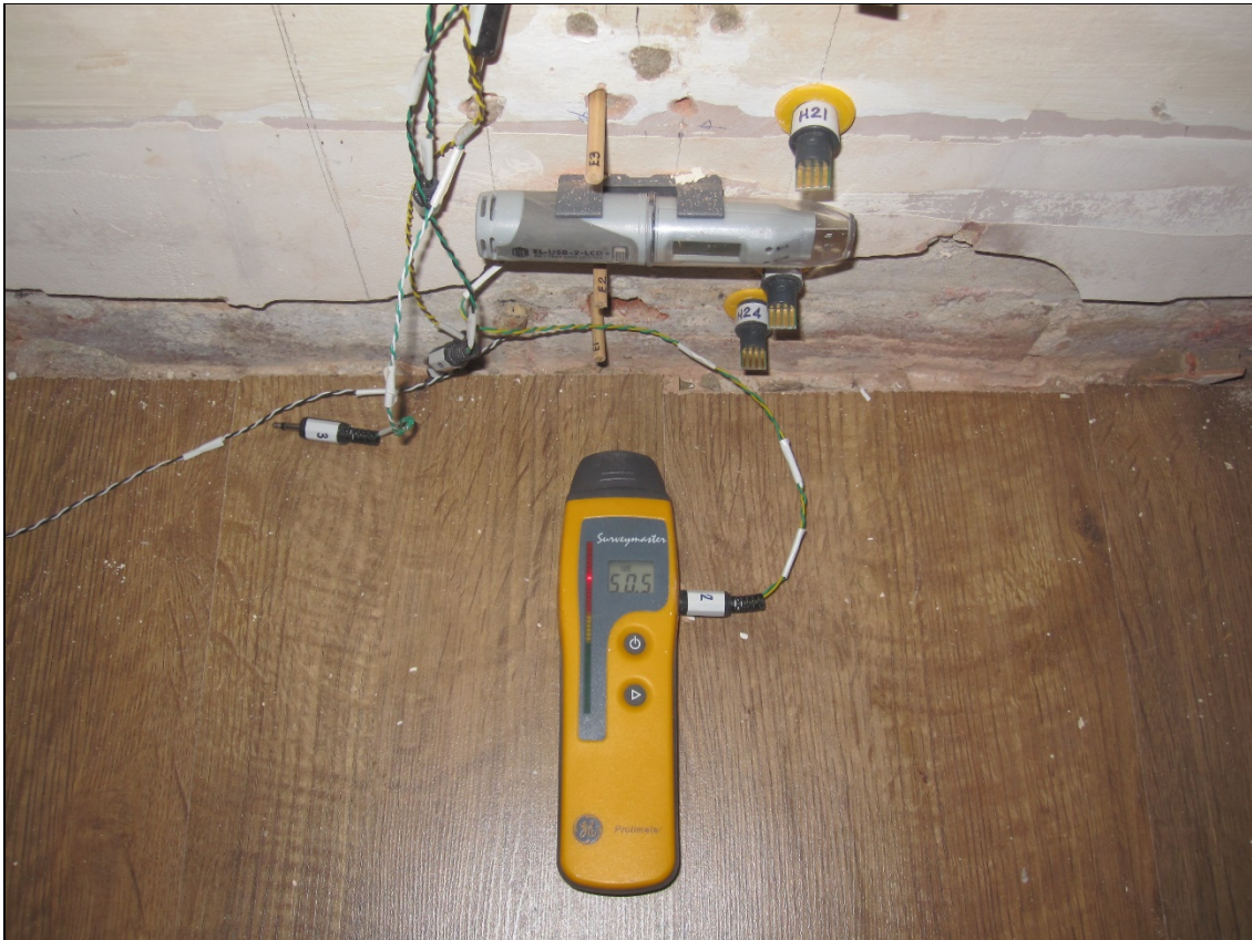
Figure 146: Panel E measure-mode reading of a Timber Probe Type 1. Timber Probes Type 1 read using the measure-mode function of the Protimeter.
