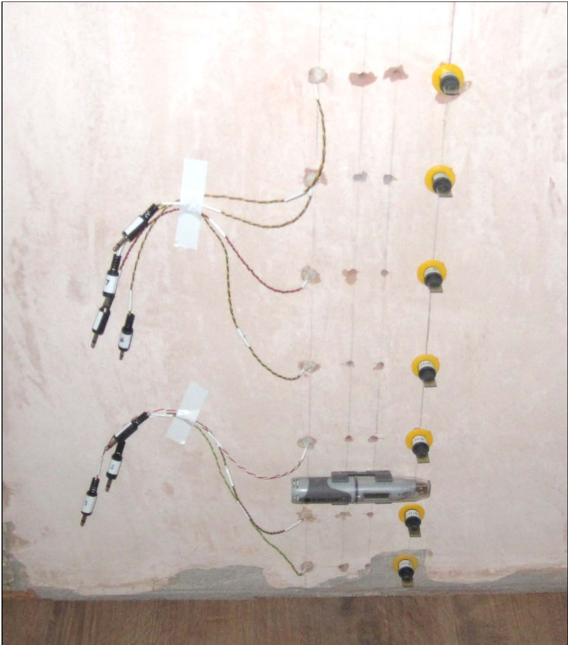
Figure 83: Panel C typical moisture measuring apparatus configuration with Hygrosticks in place.
