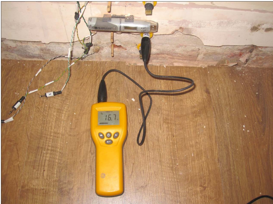
Figure 45: Protimeter MMS meter reading a Hygrostick inserted into a Humidity Sleeve embedded in a masonry wall.
