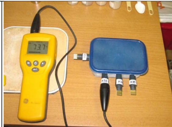
Figure 55: Hygrostick batch testing apparatus with Protimeter MMS meter attached.
