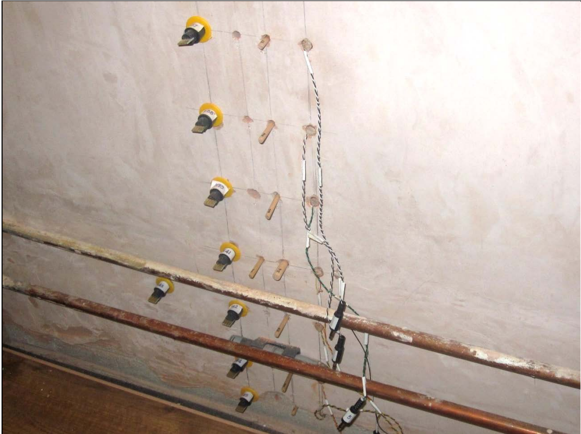
Figure 100: Panel B illustrating final configuration of the moisture measuring apparatus.
