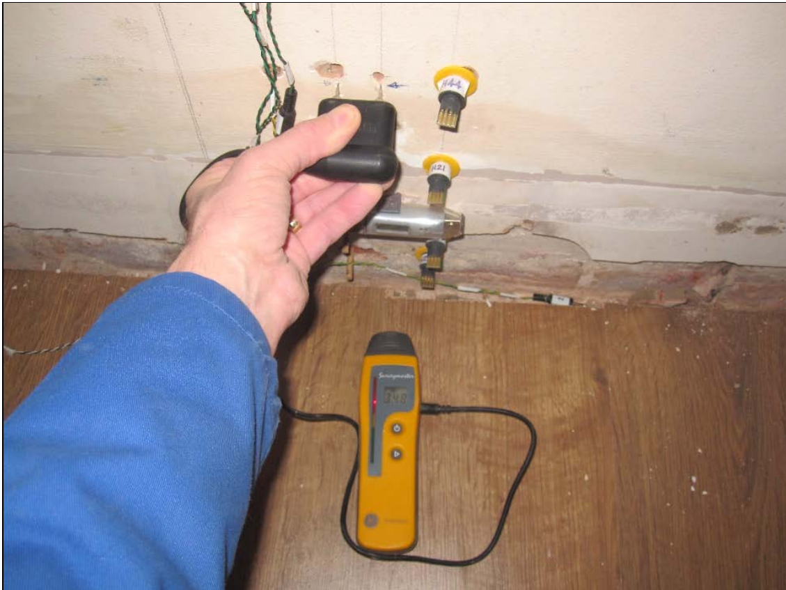
Figure 128: Panel E Protimeter measure-mode function using the Heavy Duty Probe.
