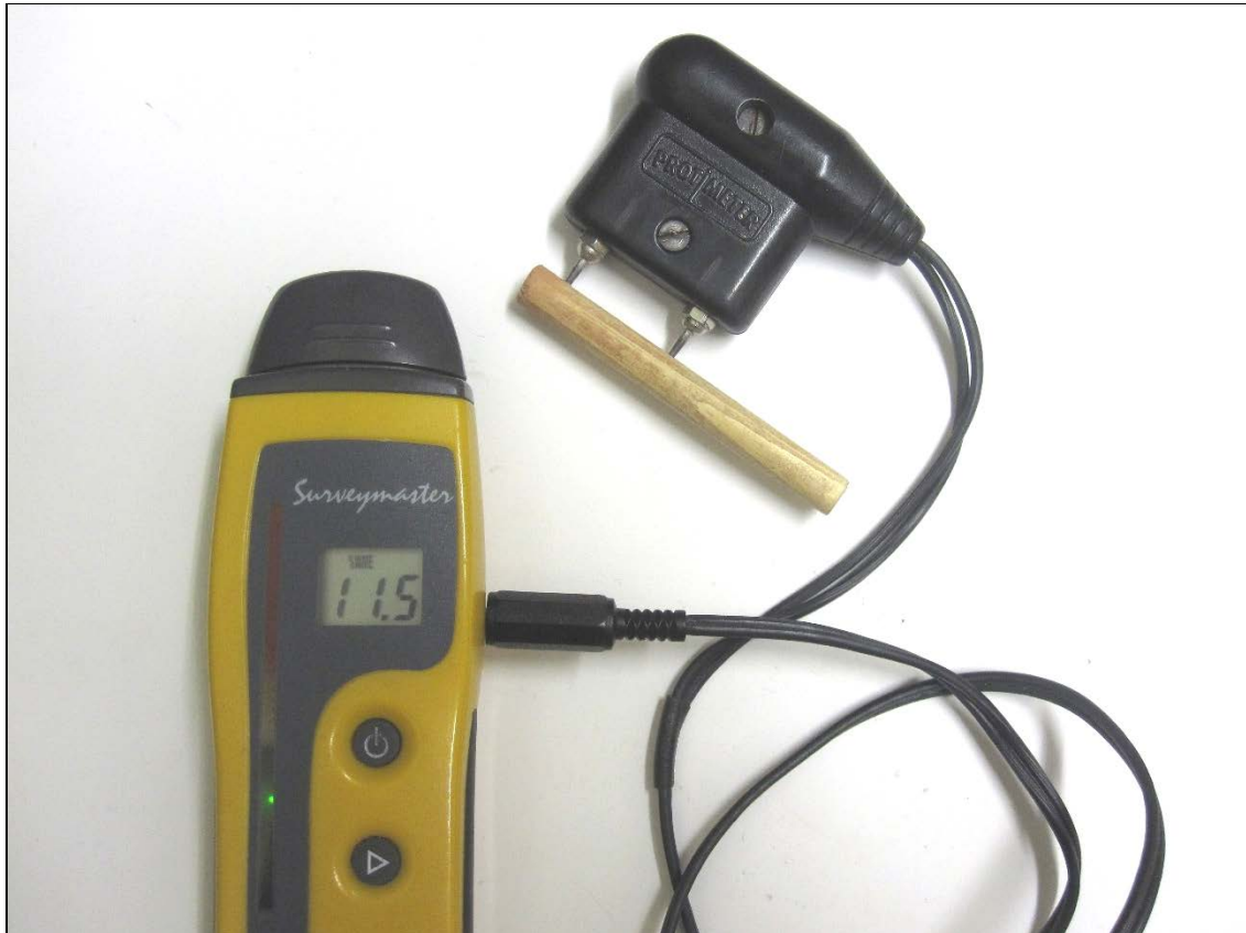
Figure 97: 9 mm diameter plain softwood dowel undergoing reading using the Protimeter measure-mode function.
