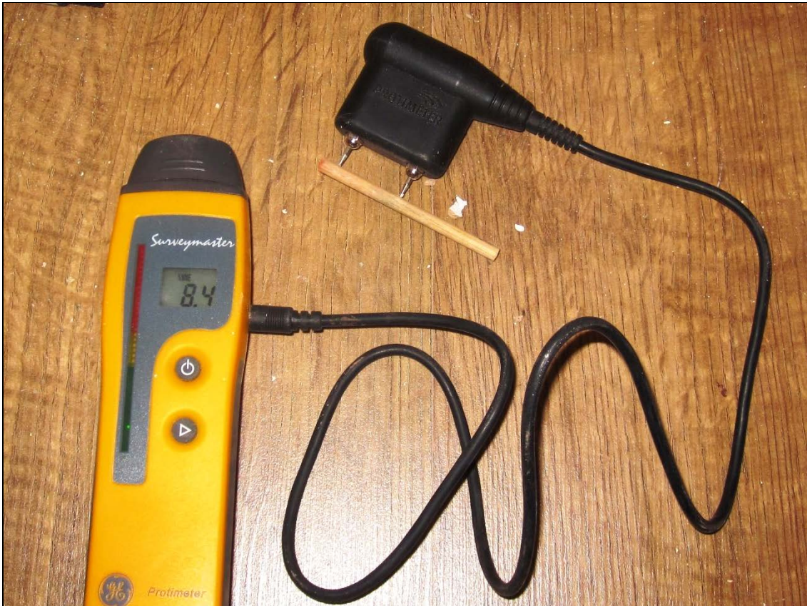
Figure 99: 5 mm diameter plain hardwood dowel undergoing reading using the Protimeter measure-mode function.
