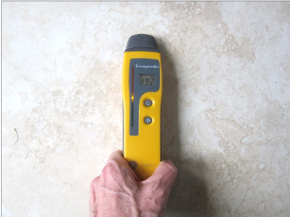
Figure 43: Protimeter Surveymaster meter: search-mode function.
