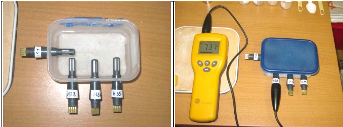
Figure 54: Hygrostick batch testing apparatus shown without lid.
