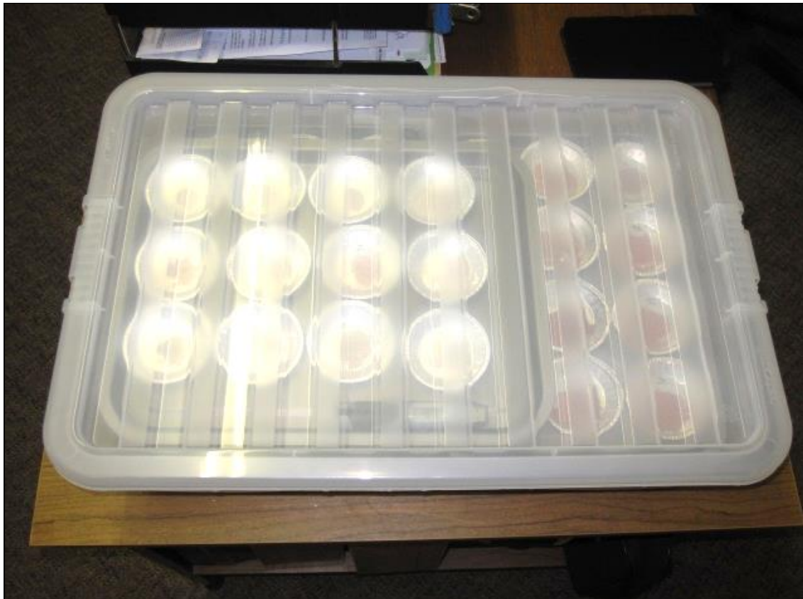
Figure 39: 75.0% relative humidity container for large batch processing.
