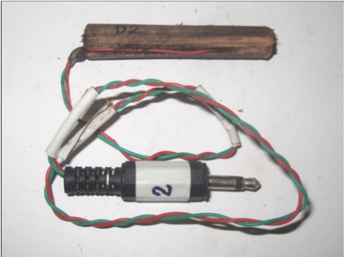
Figure 103: Timber Probe Type 1 reference D2 following removal from Panel D.
