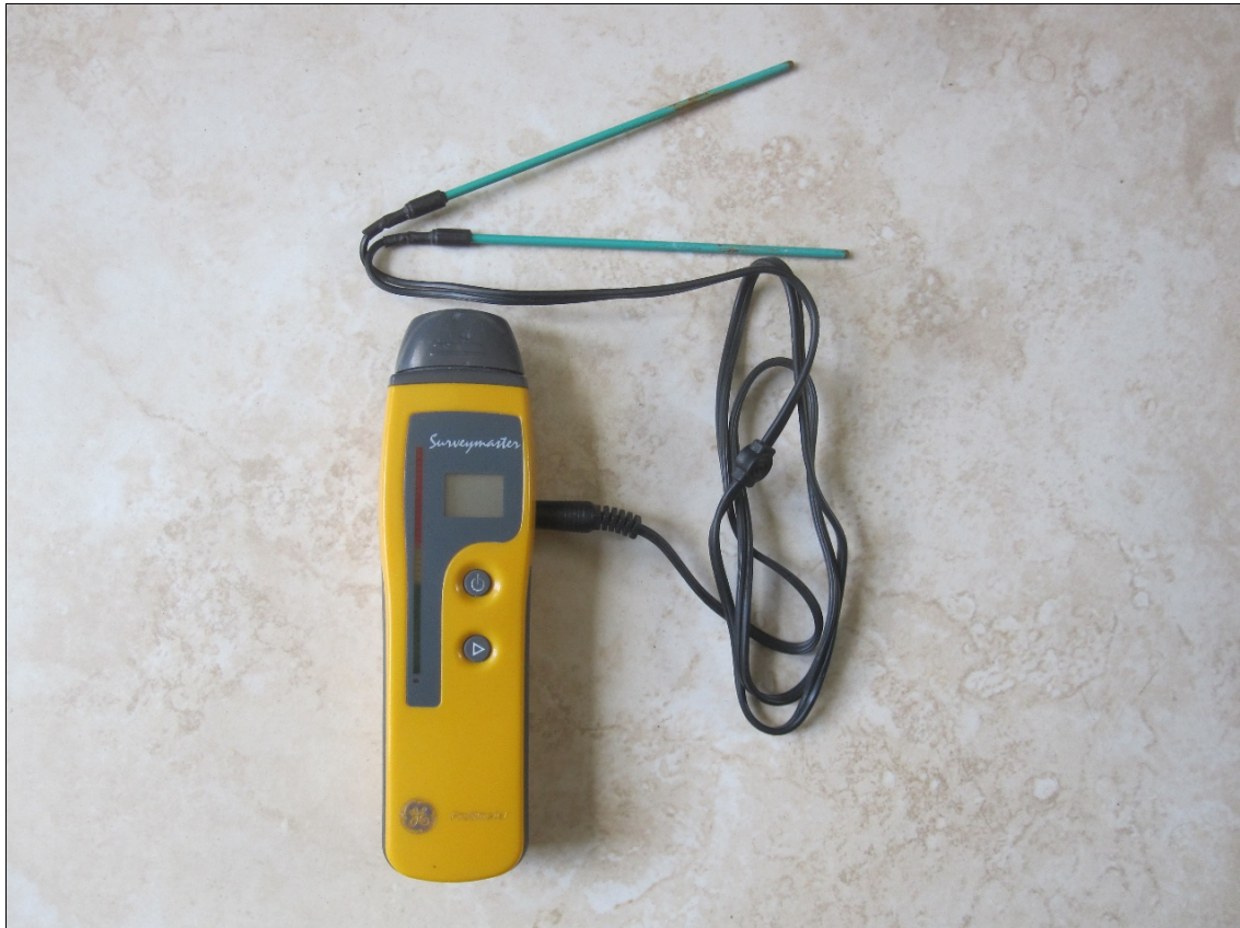
Figure 42: Protimeter Surveymaster meter: Deep Wall Probes attached.
