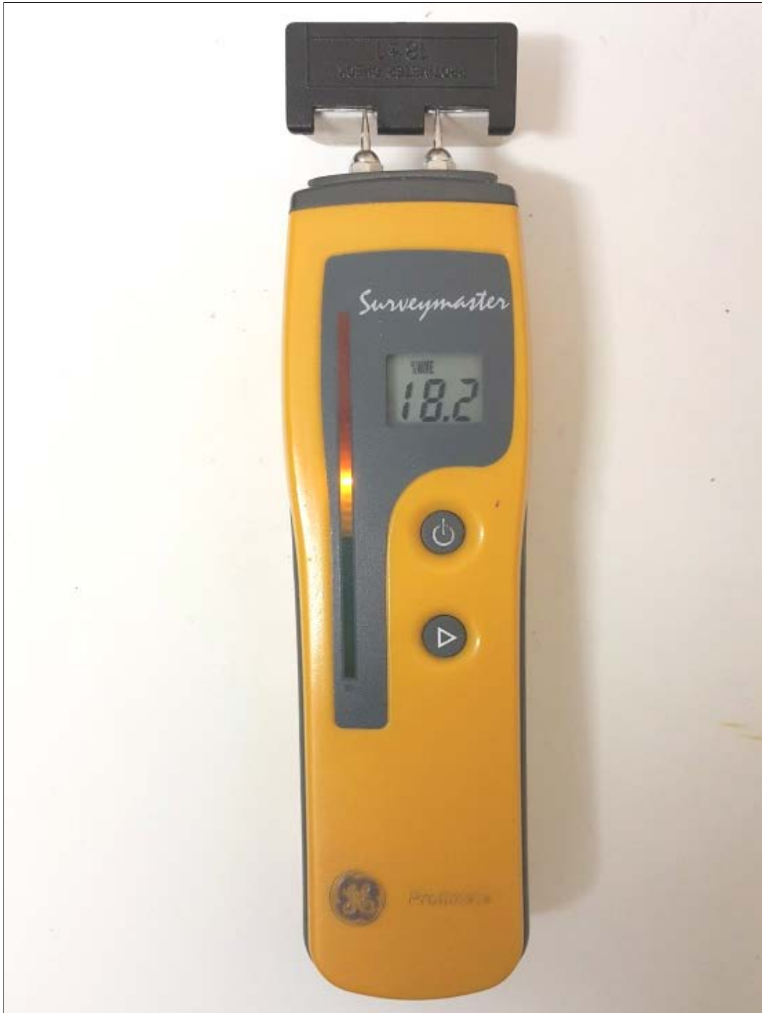
Figure 53: Protimeter Surveymaster meter: calibration using Calcheck tool.
