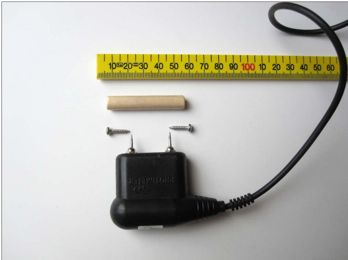
Figure 51: Timber Probes Type 1 & 2: screw configuration.
