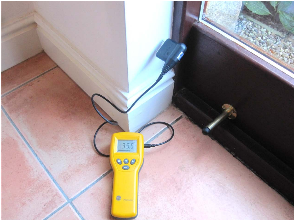
Figure 40: Protimeter MMS meter: measure-mode function using the Heavy Duty Probe.
