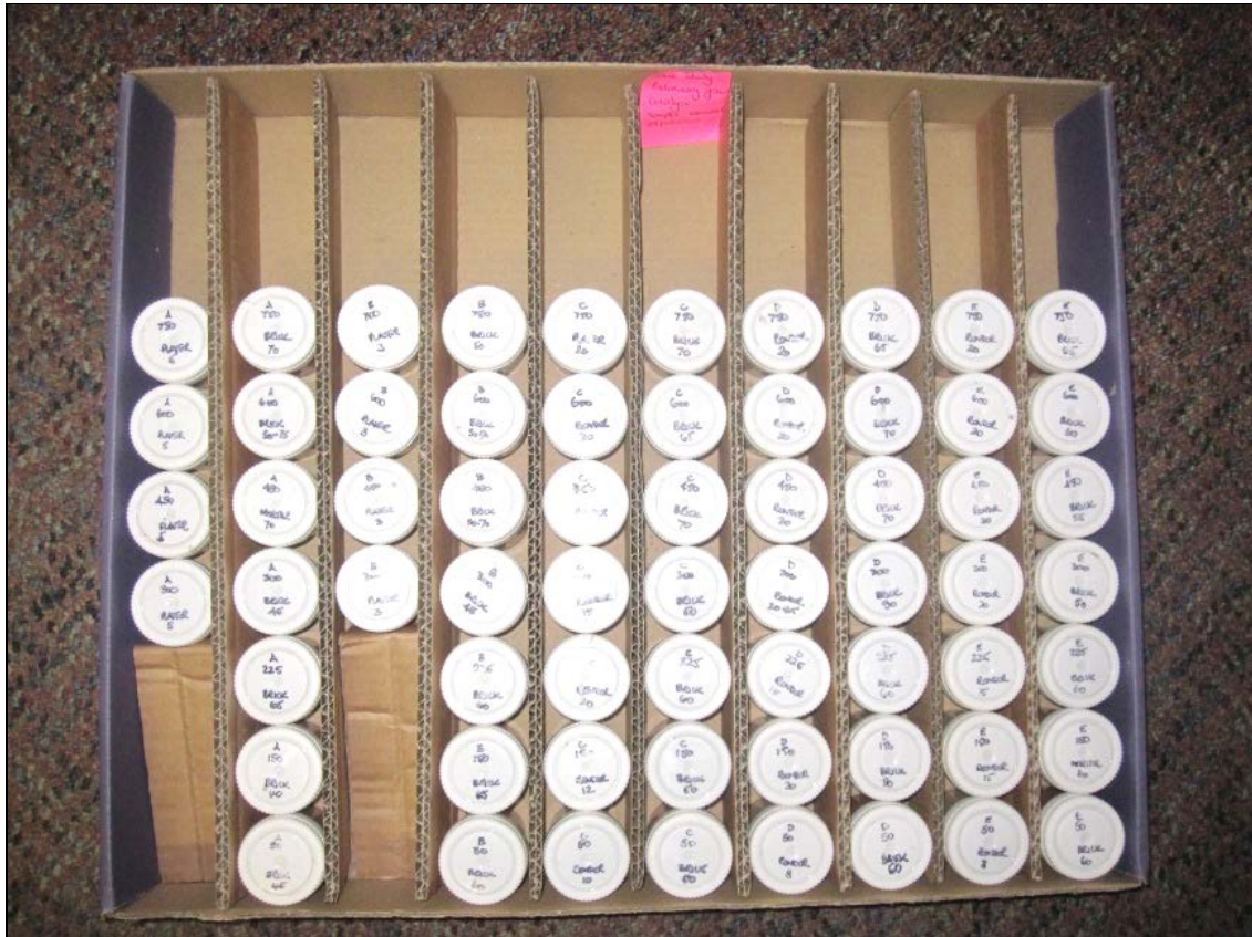
Figure 63: Samples obtained for the Stage 2 moisture analysis placed in individual air tight containers ready for processing.
