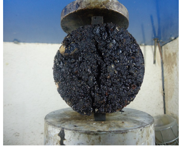
b. Failed specimen
