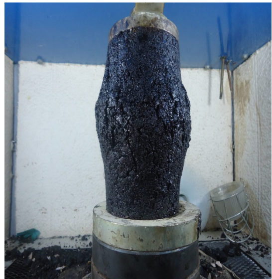
b. Failed specimen
