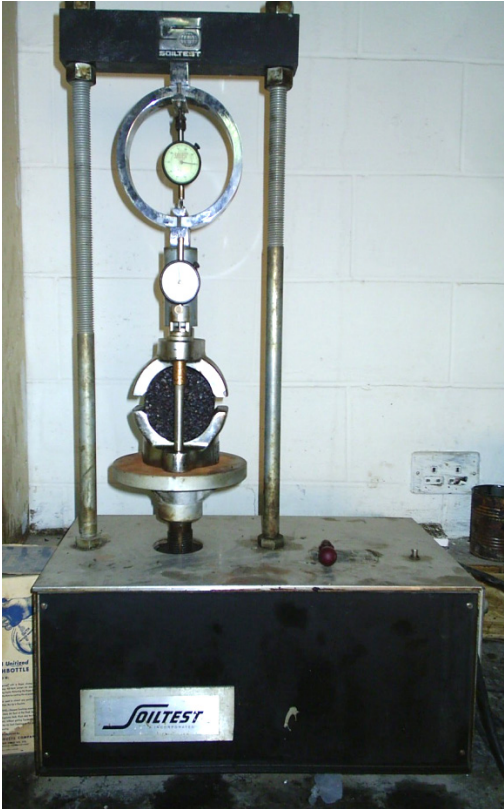
Figure (3-7) Marshall Apparatus for Determination of Stability and Flow
