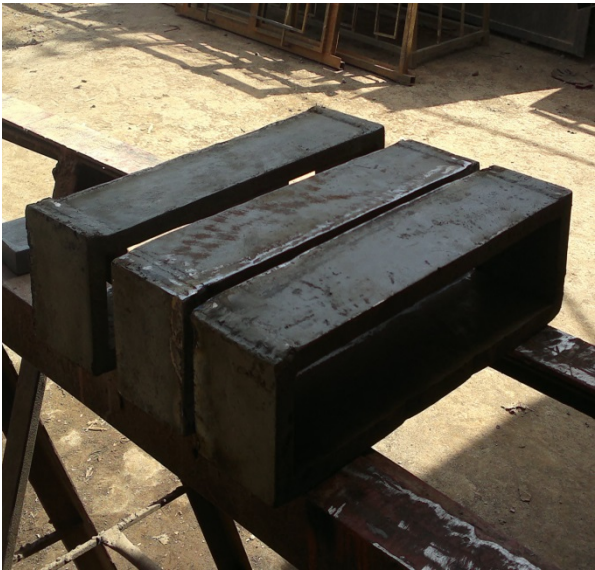
a. Flexural beam specimen molds
