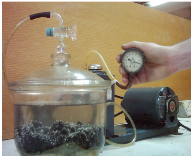
Figure (3-8) Maximum Specific Gravity Calculation for Asphalt Concrete Specimen
