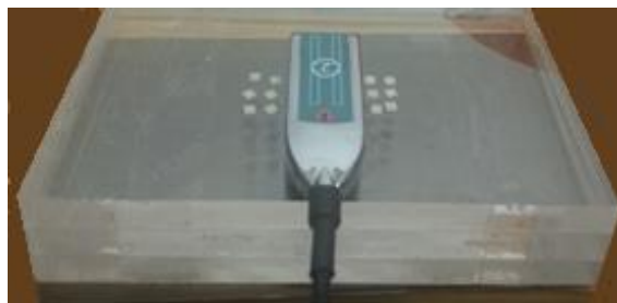
Figure (5-8) Demonstrates the TLD calibration process against the Unfors solid state dosimeter on three Perspex slabs.
