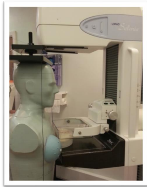
Figure (5-14) ATOM and CC breast phantoms on FFDM system in CC position.
