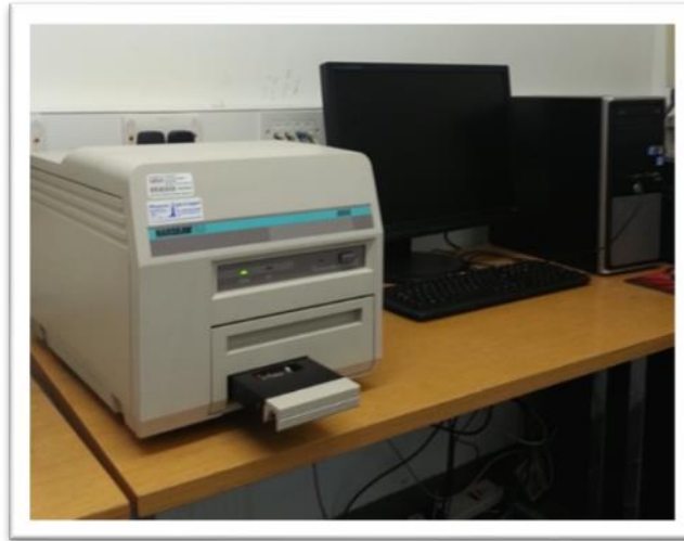
Figure (5-3) Shows the TLD reading system.
