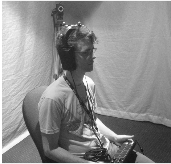
Figure 5.6: A picture demonstrating how listeners participated in the headphone transparency behavioural study. The response device can be seen on the participants lap. Reflective markers are visible mounted to the top of the headphones and one of the four tracking cameras can be seen in the background.
