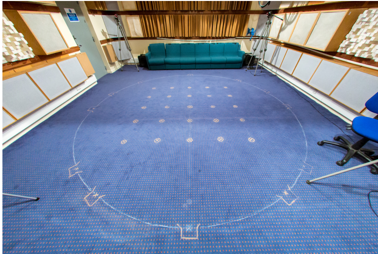
Figure 4.2: Photo of the SBSBRIR measurement positions. Markings on the floor indicate the 0.5m resolution measurement grid and loudspeaker positions relative to the size of the listening room. The photo graph is taken from position X = 3\text{m} , Y = 0\text{m} .
