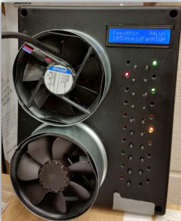
Figure 4.26: ASPEC mk2 with purpose built illuminated micro switch Human Machine Interface
