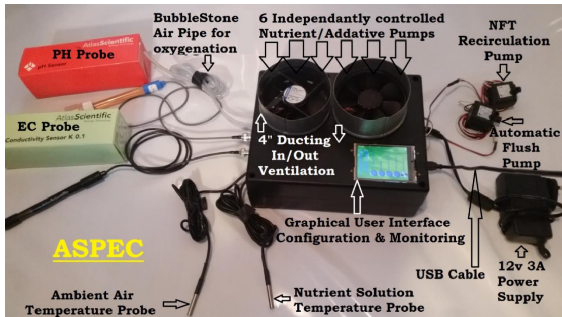
Figure 4.32: ASPEC & Additional complementary hardware layout
