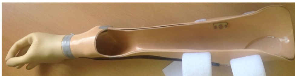
FIGURE 5 | Prosthesis simulator for use with anatomically intact subjects. The socket is designed to fit over the forearm and fist. Straps allow the socket to be tightened to the persons arm. It is not possible to tailor electrode placement to each person.
