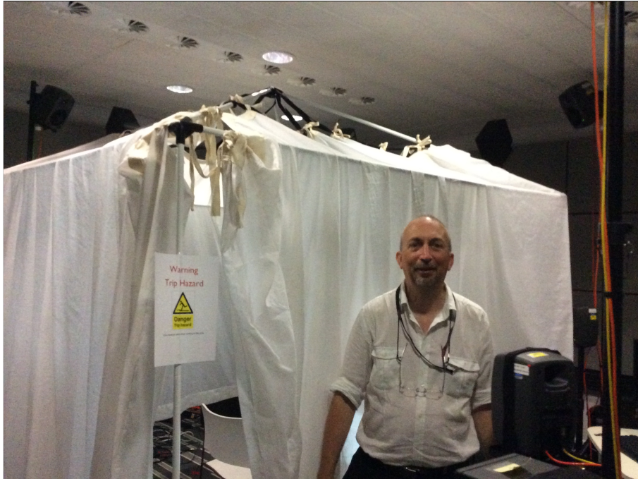
Figure 4.7: The listening test set up, with curtain to obscure the loudspeaker placement. One of the expert listeners standing aside of the rear right loudspeaker
