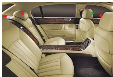
FIGURE 7.7: Cancellation zones at the three passengers headrest marked with. ● and uncontrolled zone at the driver's headrest with. ●
