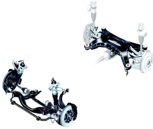
FIGURE 6.8: The locations of the accelerometers in the vehicle structure. ■: One dimensional accelerometers.
