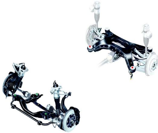
FIGURE 6.31: The locations of the accelerometers in the vehicle structure. ■: Two DoF reference signals. ■: One direction acceleration signal.
