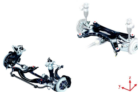
FIGURE 6.2: The locations of the accelerometers in the vehicle structure and the directions of the reference signals. ■: One direction.
