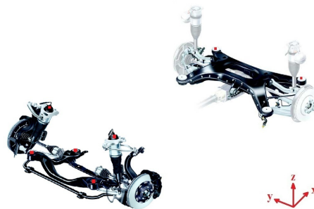
FIGURE 6.25: The locations of the accelerometers in the vehicle structure and the DoF of the reference signals. ●: Three DoF. ■: One DoF.
