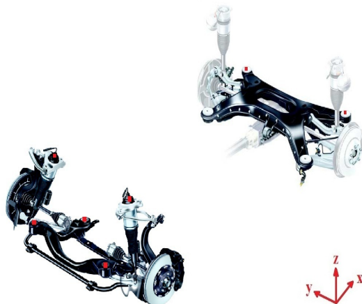
FIGURE 6.23: The locations of the accelerometers in the vehicle structure. ●: Tri-axial accelerometers position. ■: One dimensional accelerometers.
