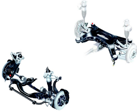
FIGURE 3.5: Accelerometer locations at front and rear axles. The two front locations are symmetrical at the front suspension and one at the rear subframe mount at the rear axle. ■: One dimensional accelerometers
