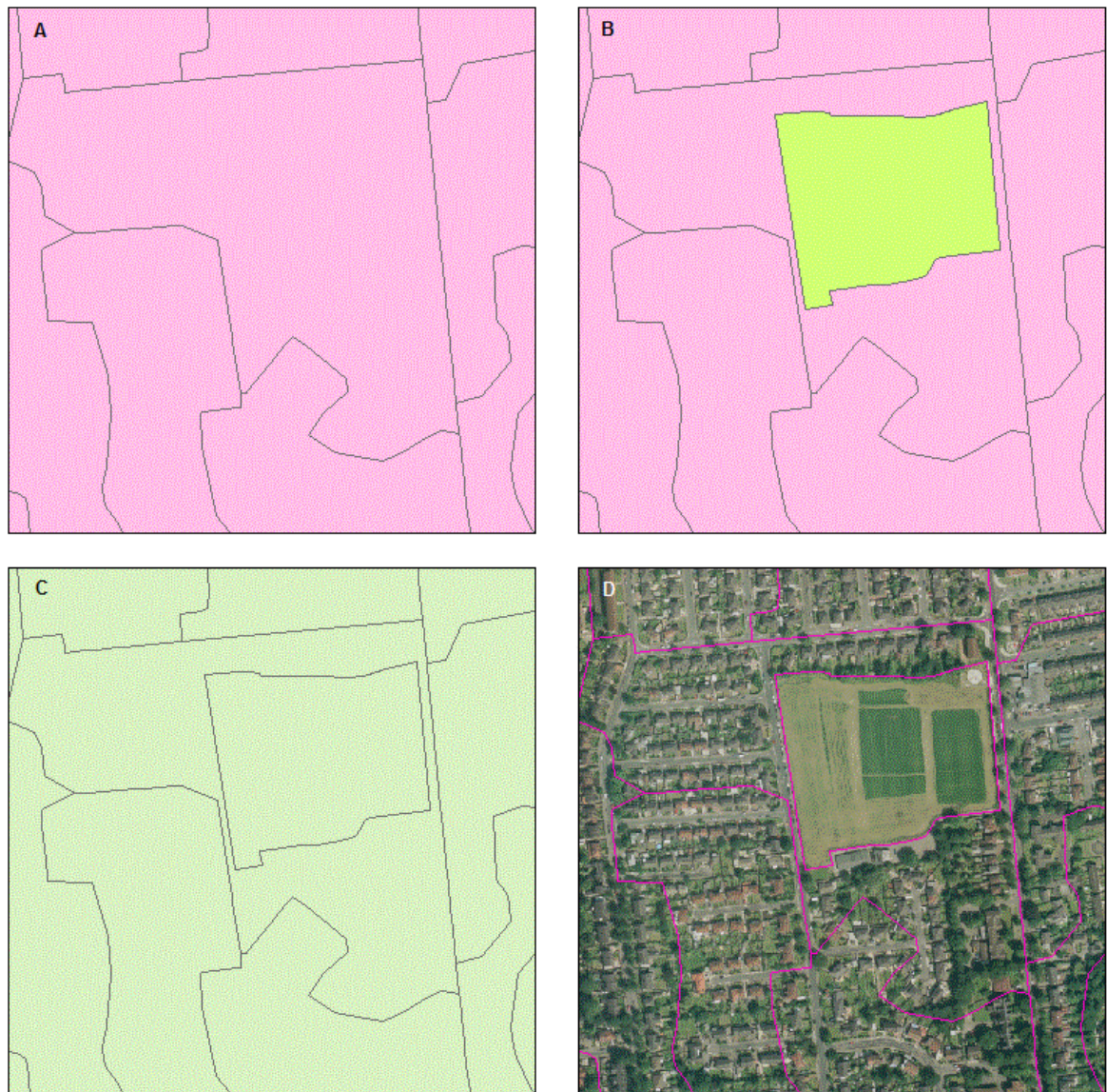
Figure 4.5. Integration of 2 ha green spaces into OA layer. (A), OA layer, (B) overlaid green spaces, (C) union function, (D) final product overlaid onto aerial photography (Landmap; The GeoInformation Group 2007).
