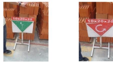
Figure 17-Pull-replenishment/production kanbans for bricks
