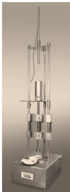
Figure 2.2 SATRA STM 479 Dynamic shock absorption test machine
