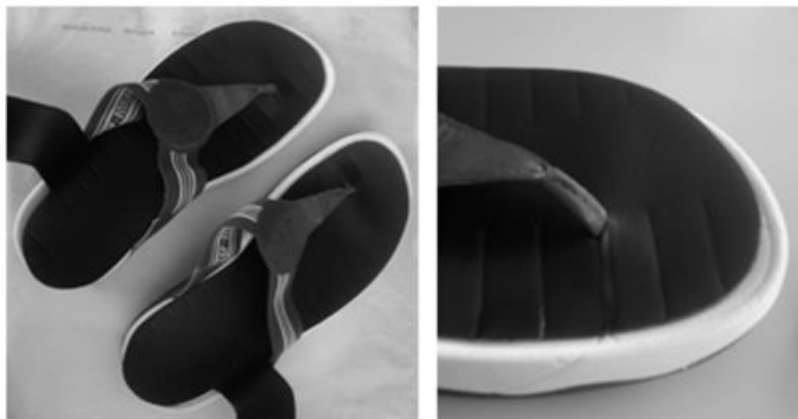
Figure 3.10 Bespoke instrumented insoles positioned and fastened with double-sided tape in the FitFlop test condition.
