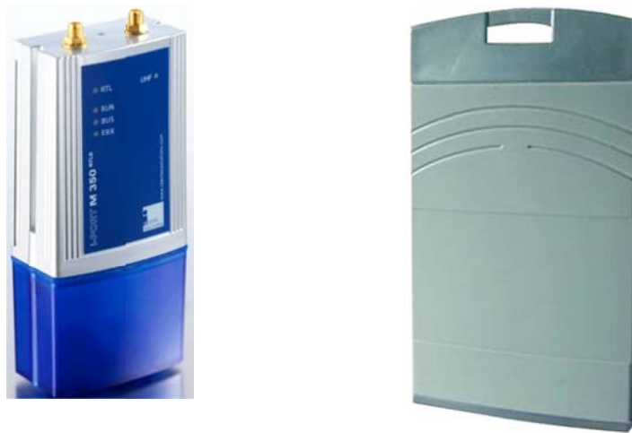
Figure 6.4: iPort-M RFID reader and ID card form factor RFID tags
