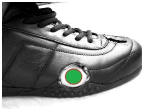
Figure 5.13: Direct skin-marking technique used for the reflective marker placement.
