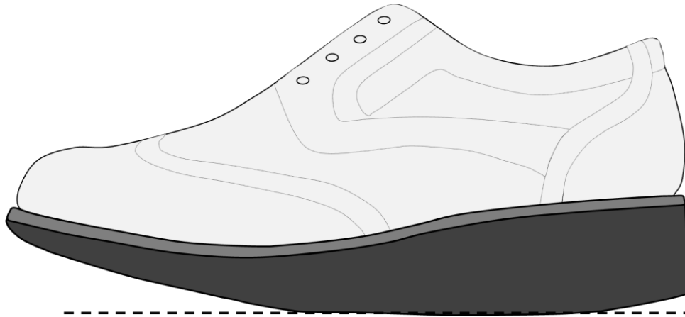
Figure 7.8: The example of estimated final design to offload the calf muscle.
