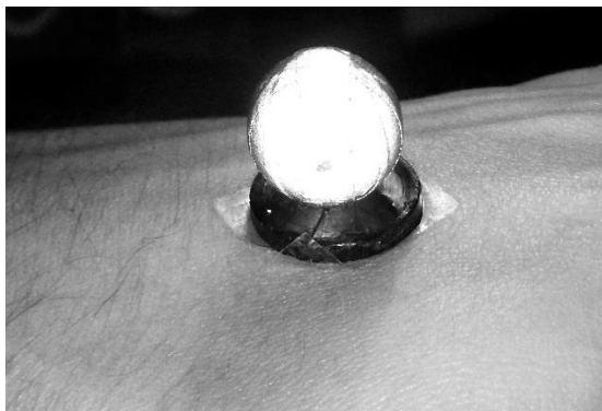
Figure 5.11: A 14 mm retroreflective marker attached to the skin using double-sided tape.
