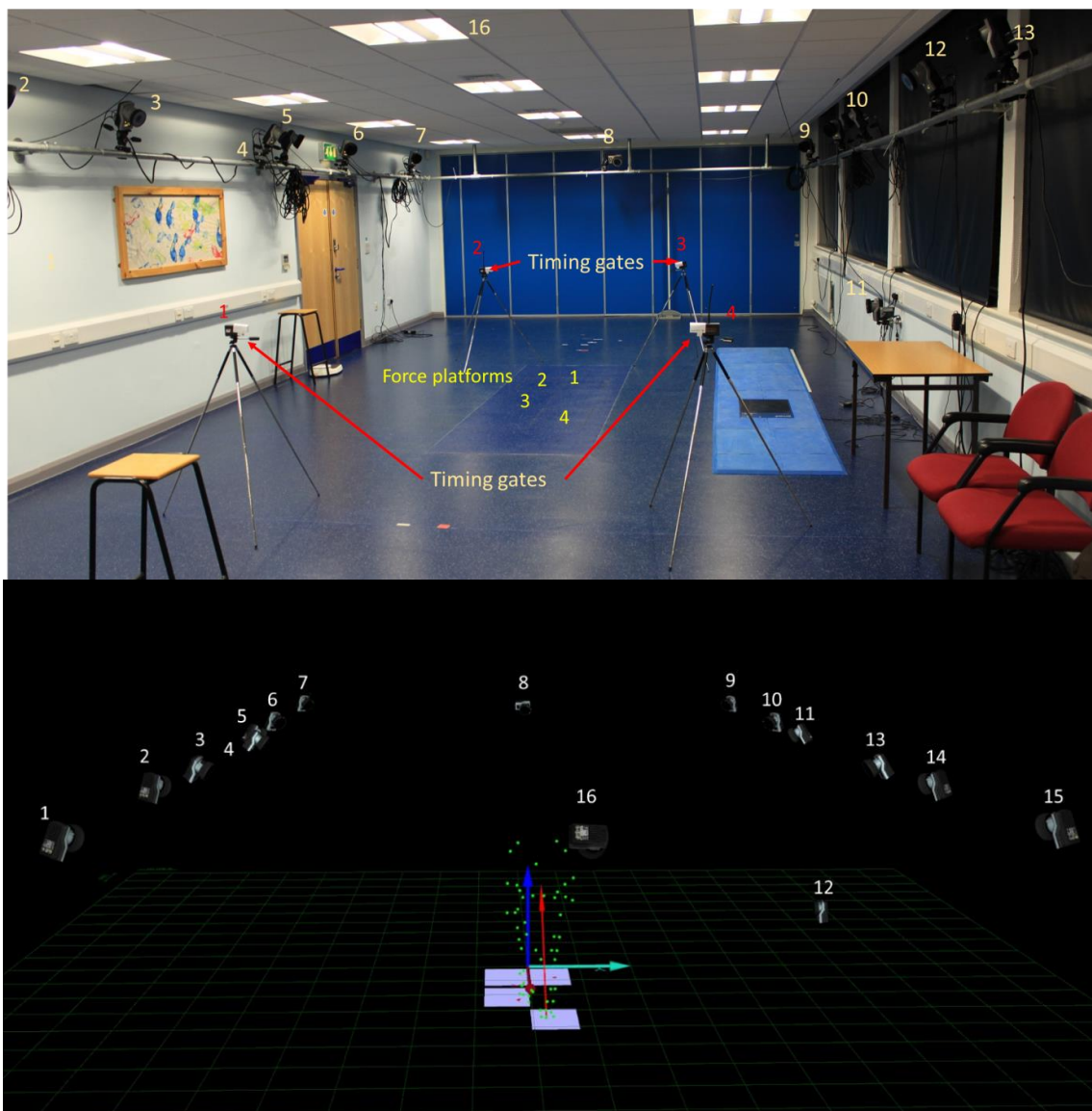
Figure 5.1: Camera set-up in the gait laboratory with an example of a typical image produced by the Qualisys software.
