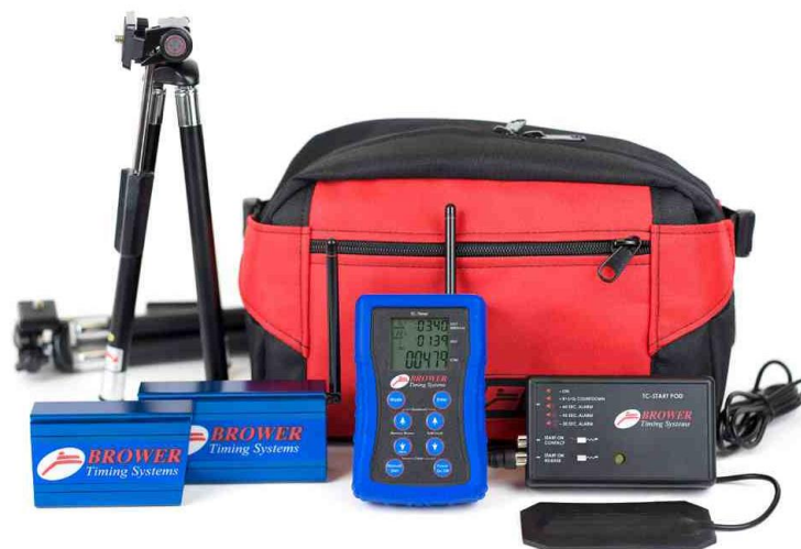
Figure 5.30: The Brower SpeedTrap II timing gate system.
