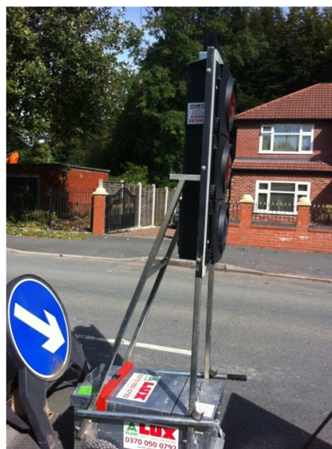
Figure A.39: Photo of the signal control equipment at temporary traffic signal
