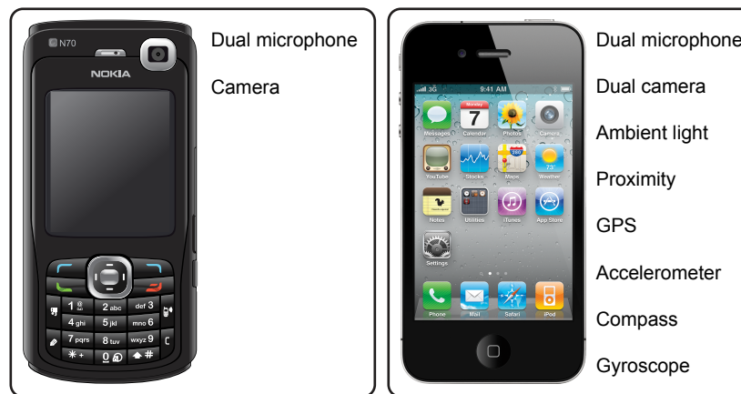
Figure 3.1: Sensor capabilities of feature phone compared to iPhone 4
