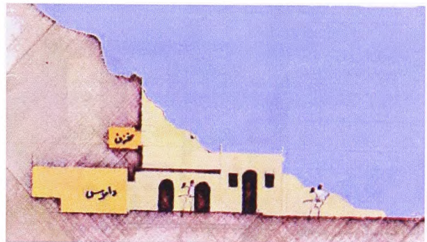
Figure 4.36: Plan and section of Alfaseal underground houses. Source: After Albakosh and Emhemed (1998)
