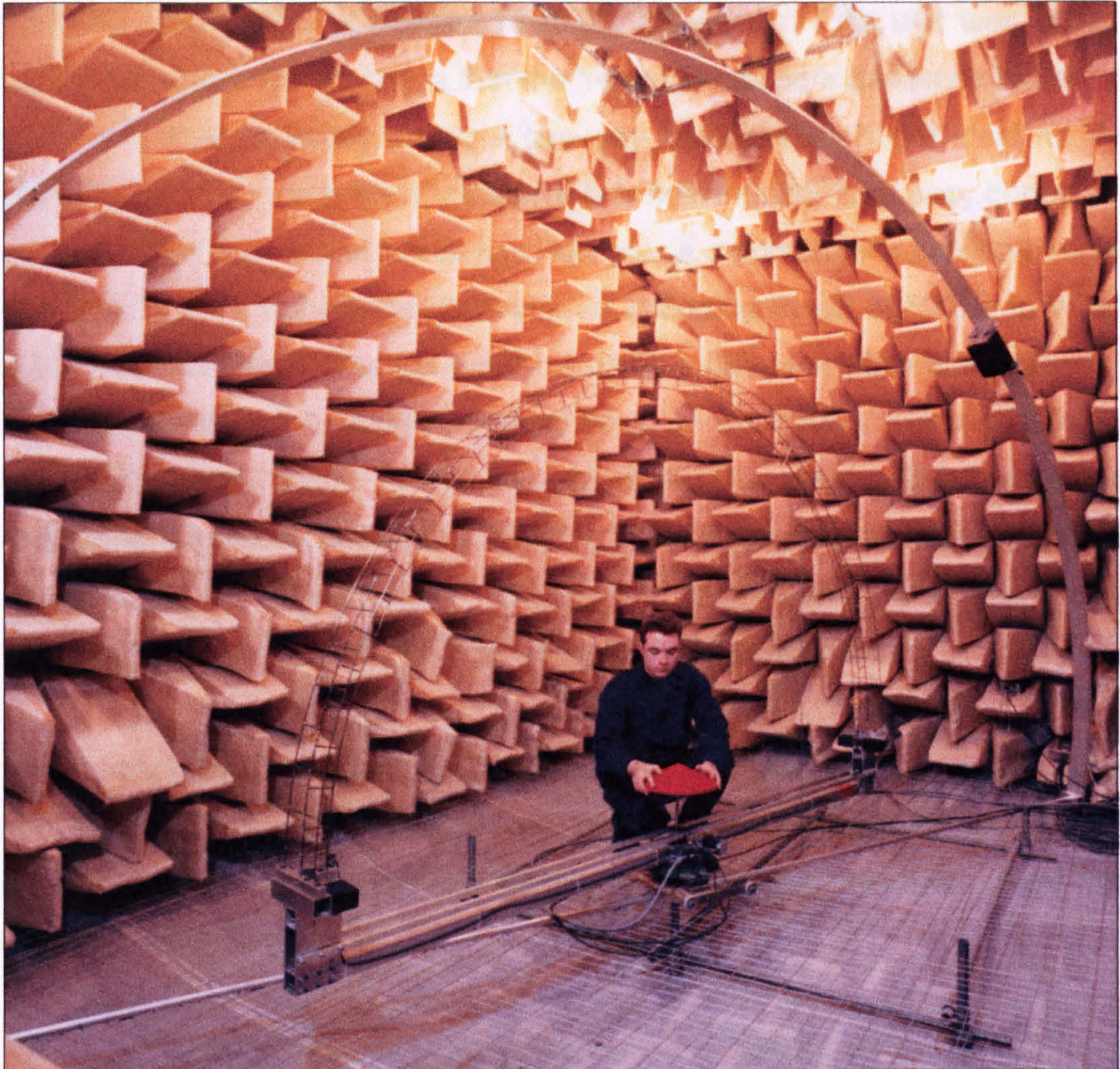
Figure 2.30: Complete apparatus for measuring three-dimensional polar responses.
