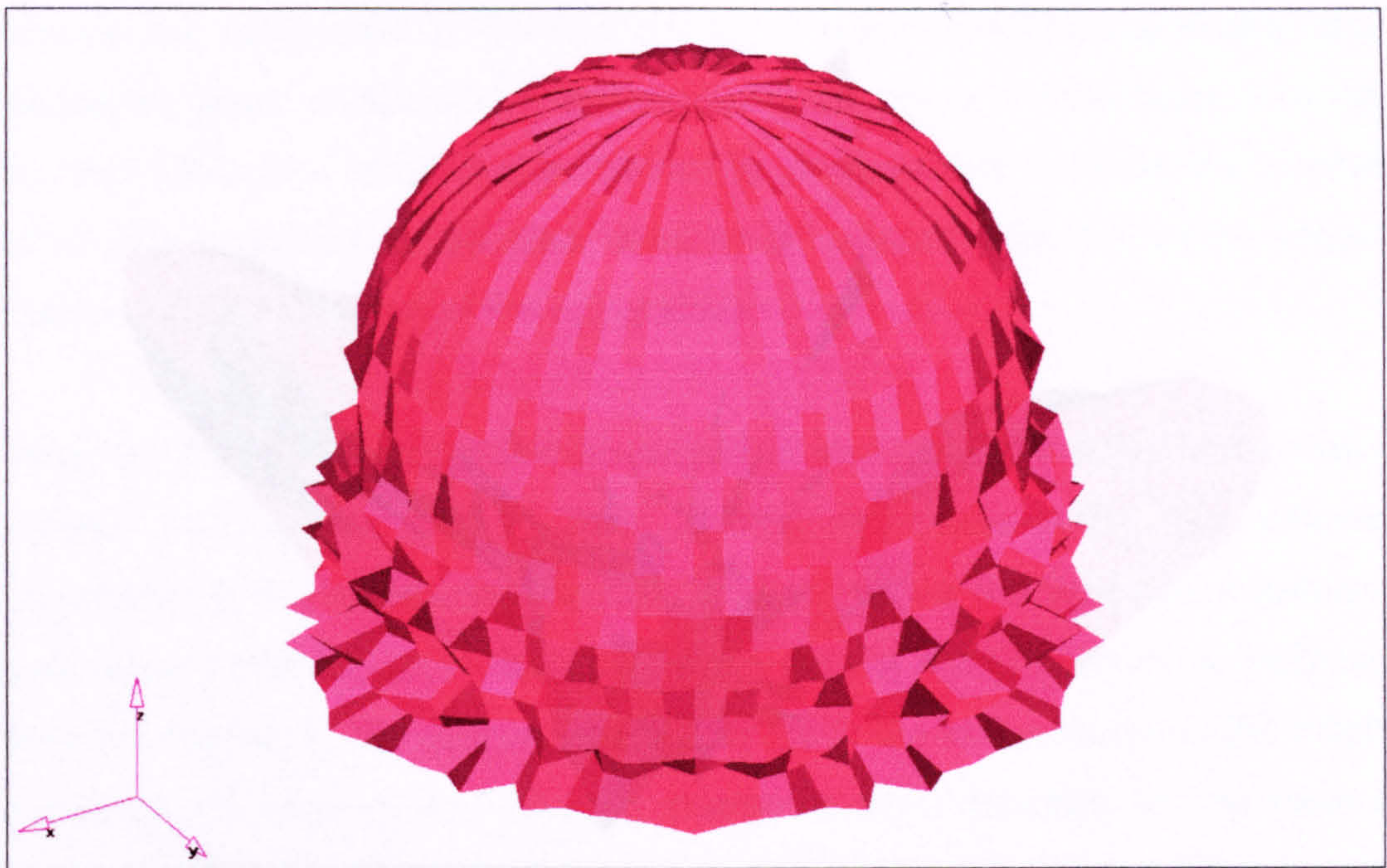
Figure 2.39: Measured 250Hz normal incidence three-dimensional polar response of the plane regular hexagon.
