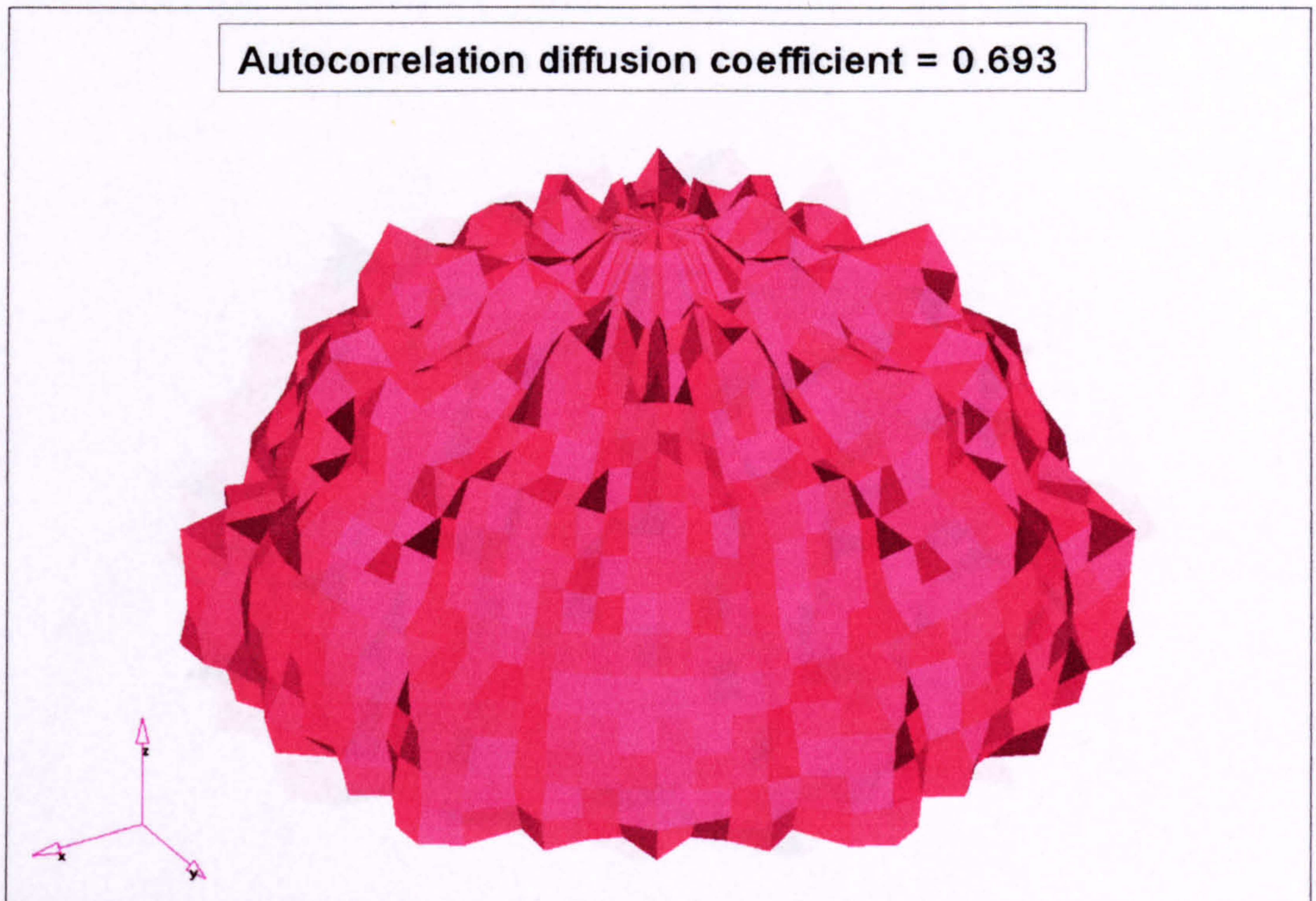
Figure 3.54: 3.15kHz normal incidence polar response of the periodic hemispheres, measured at Salford.
