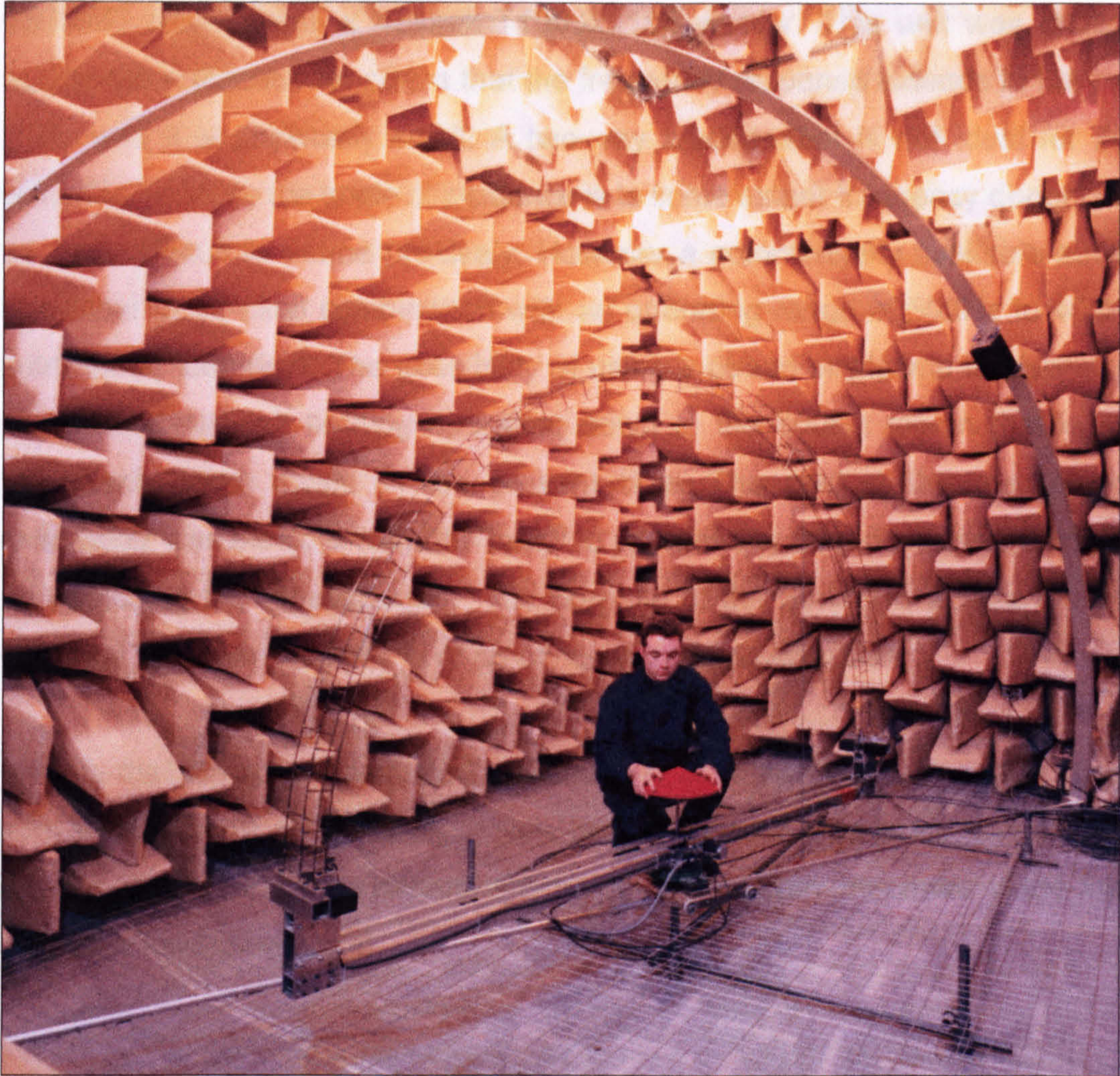
Figure 2.30: Complete apparatus for measuring three-dimensional polar responses.
