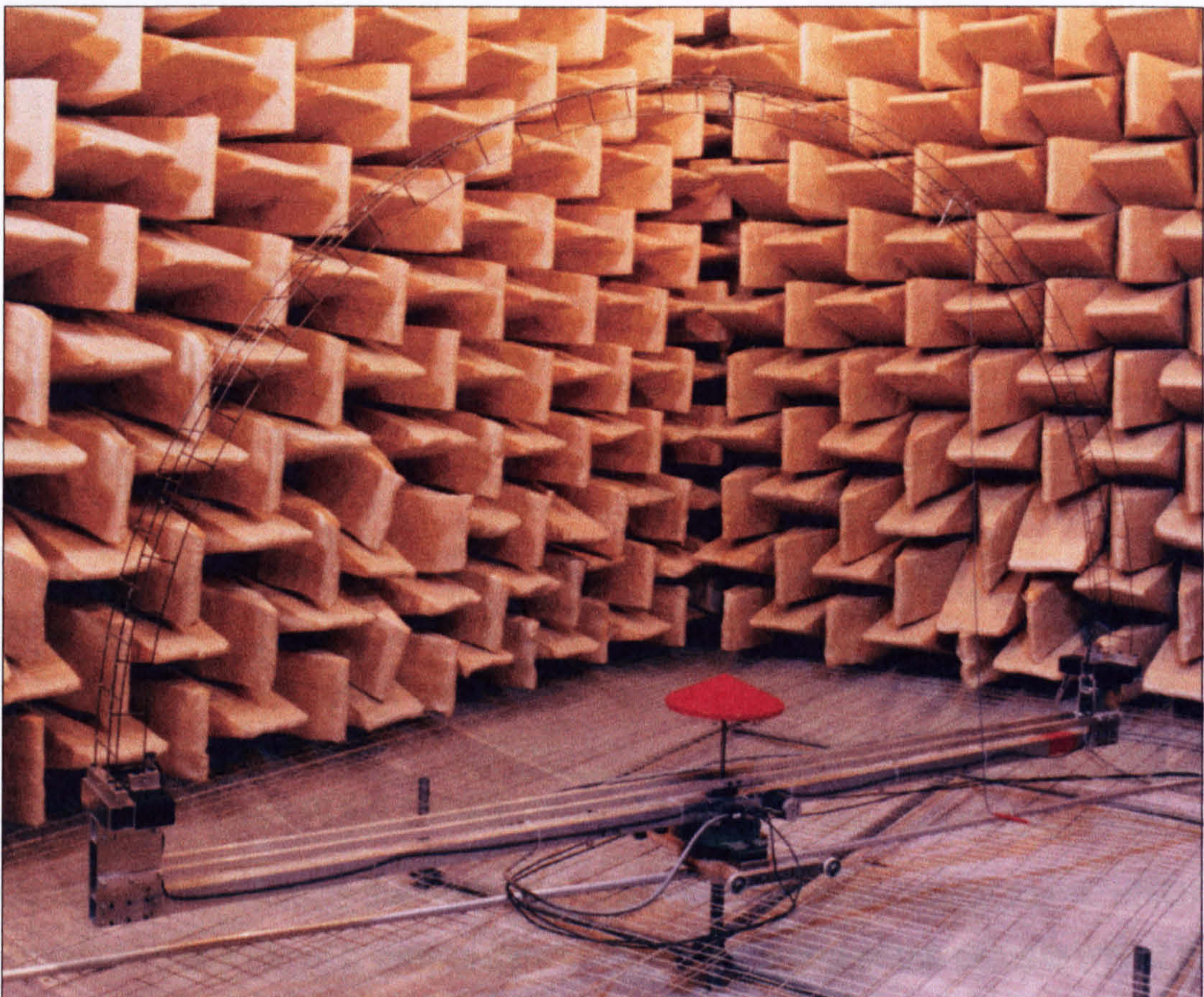
Figure 2.27: Apparatus for supporting the sample and moving the microphone over the surface of a hemisphere.
