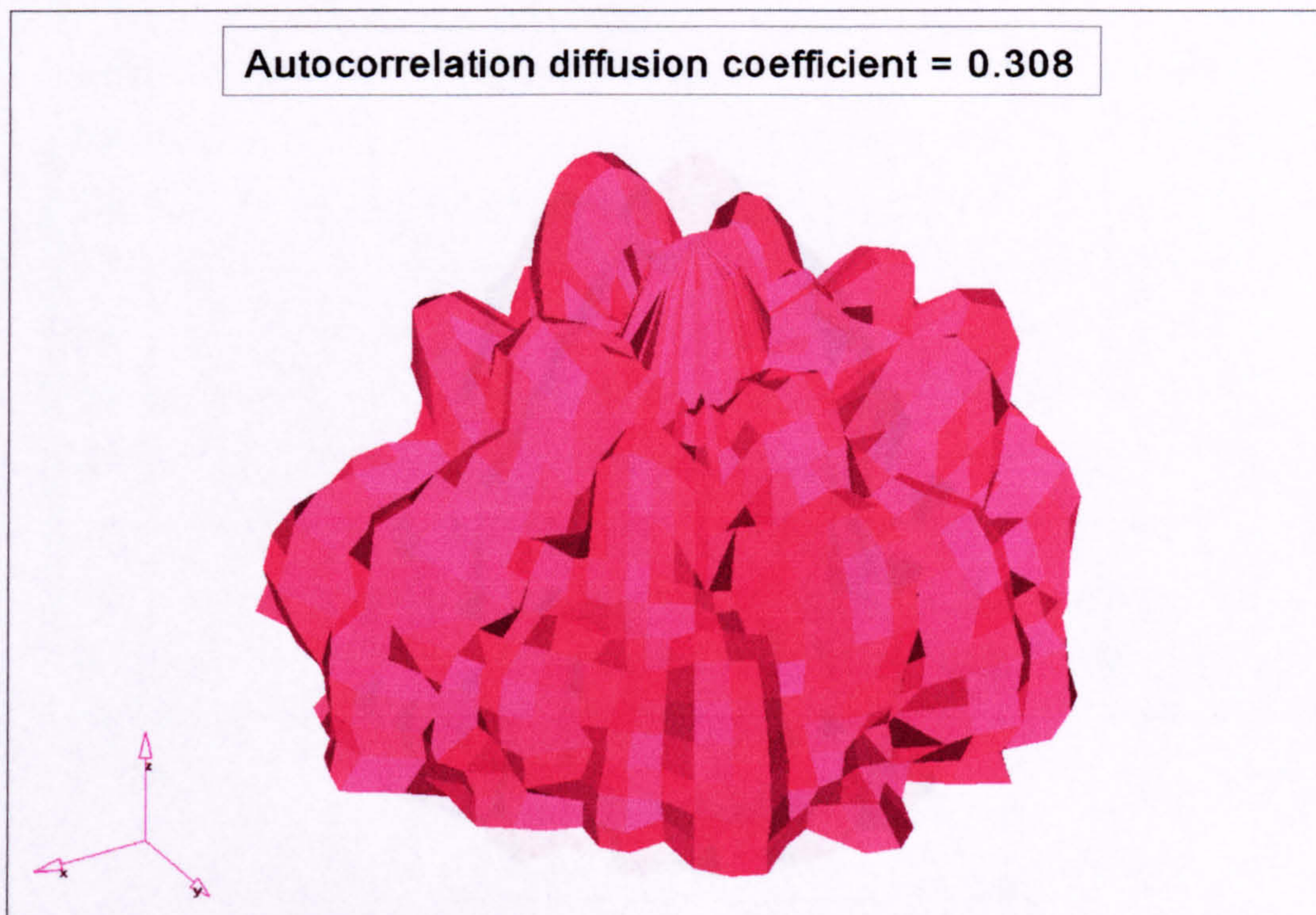
Figure 3.58: 1.6kHz normal incidence polar response of the Skyline, measured at Salford.
