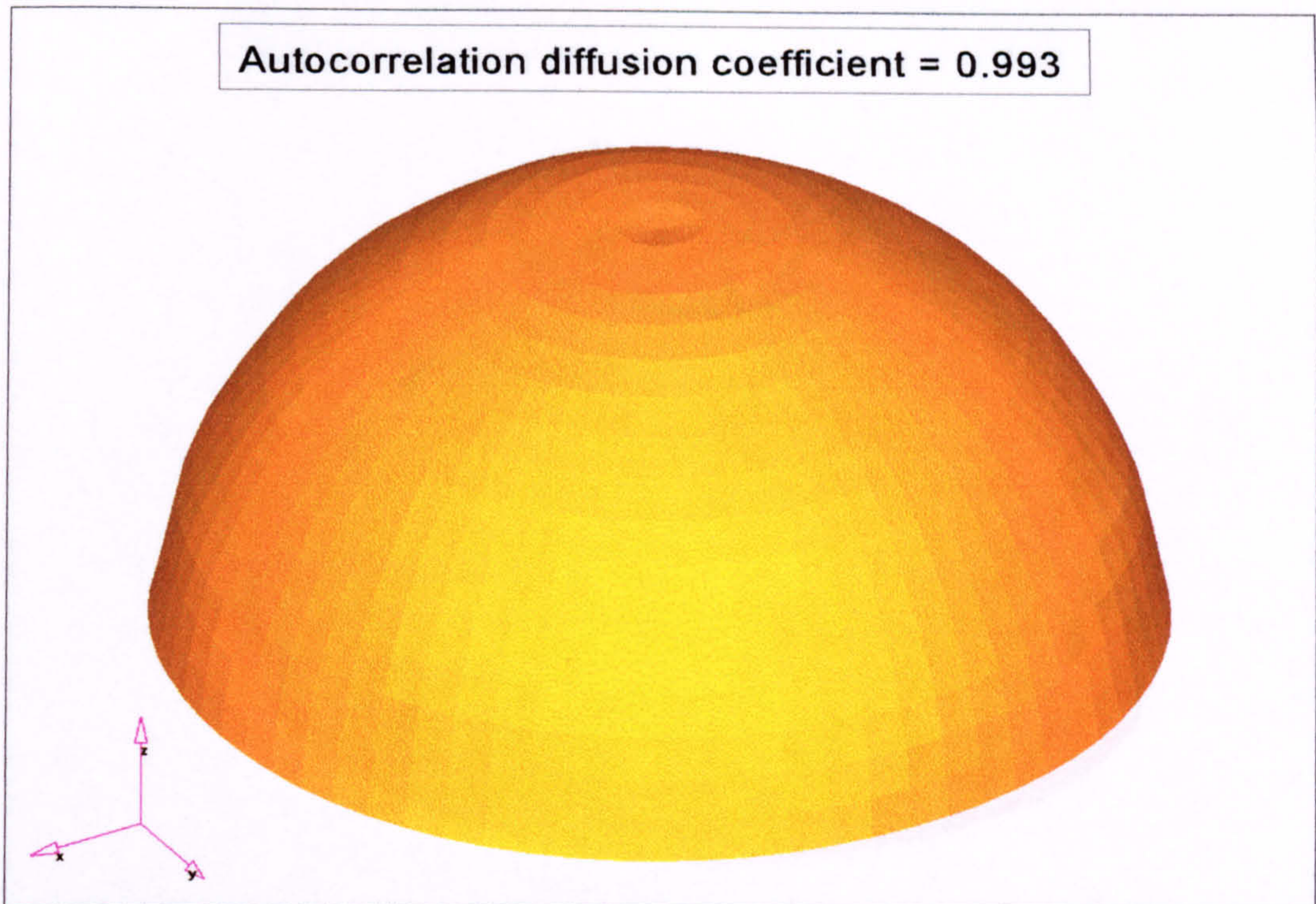
Figure 3.51: 1kHz normal incidence polar response of a small sphere, predicted using BEM.
