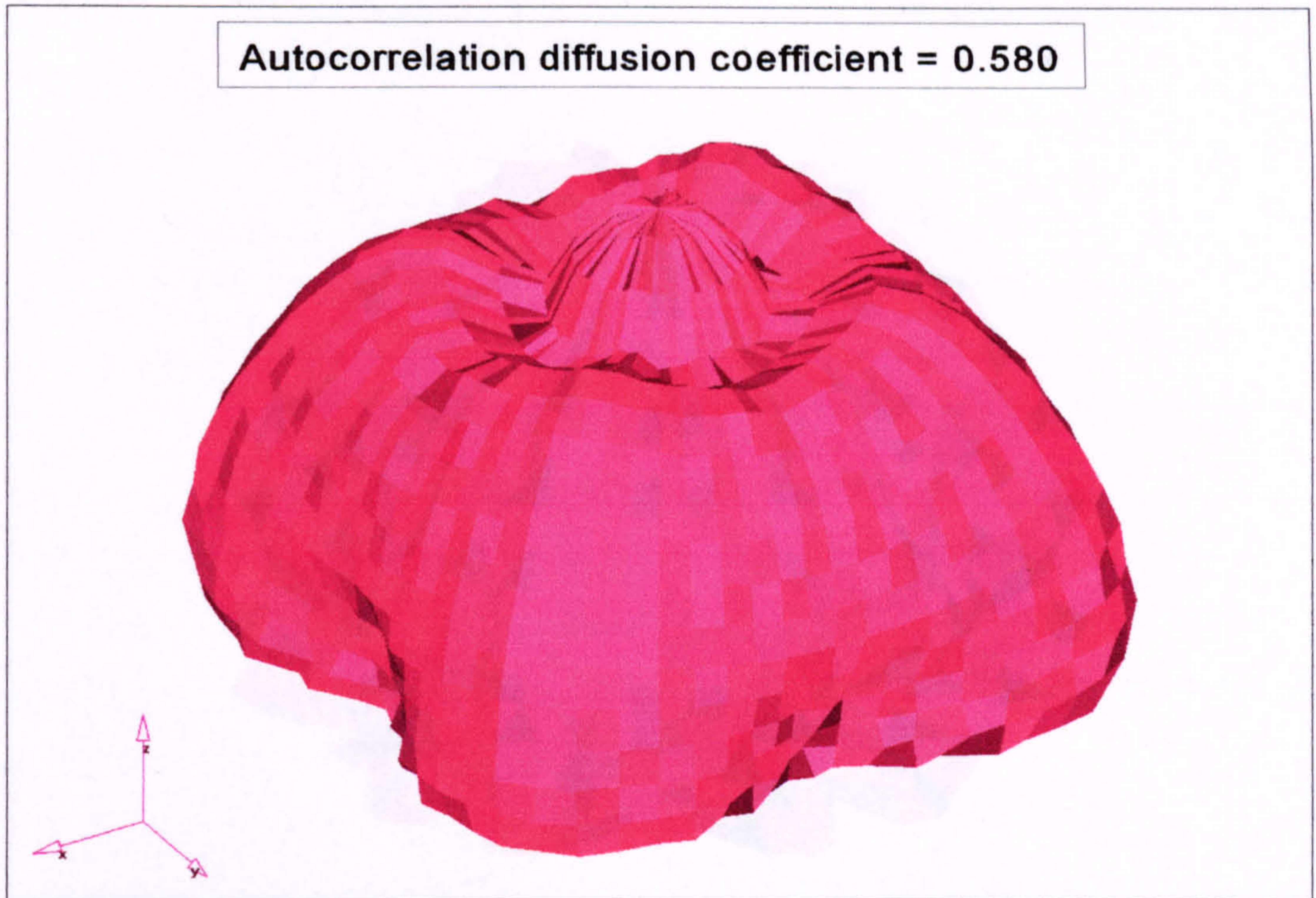
Figure 3.55: 500Hz normal incidence polar response of the square-based pyramid, measured at Salford.
