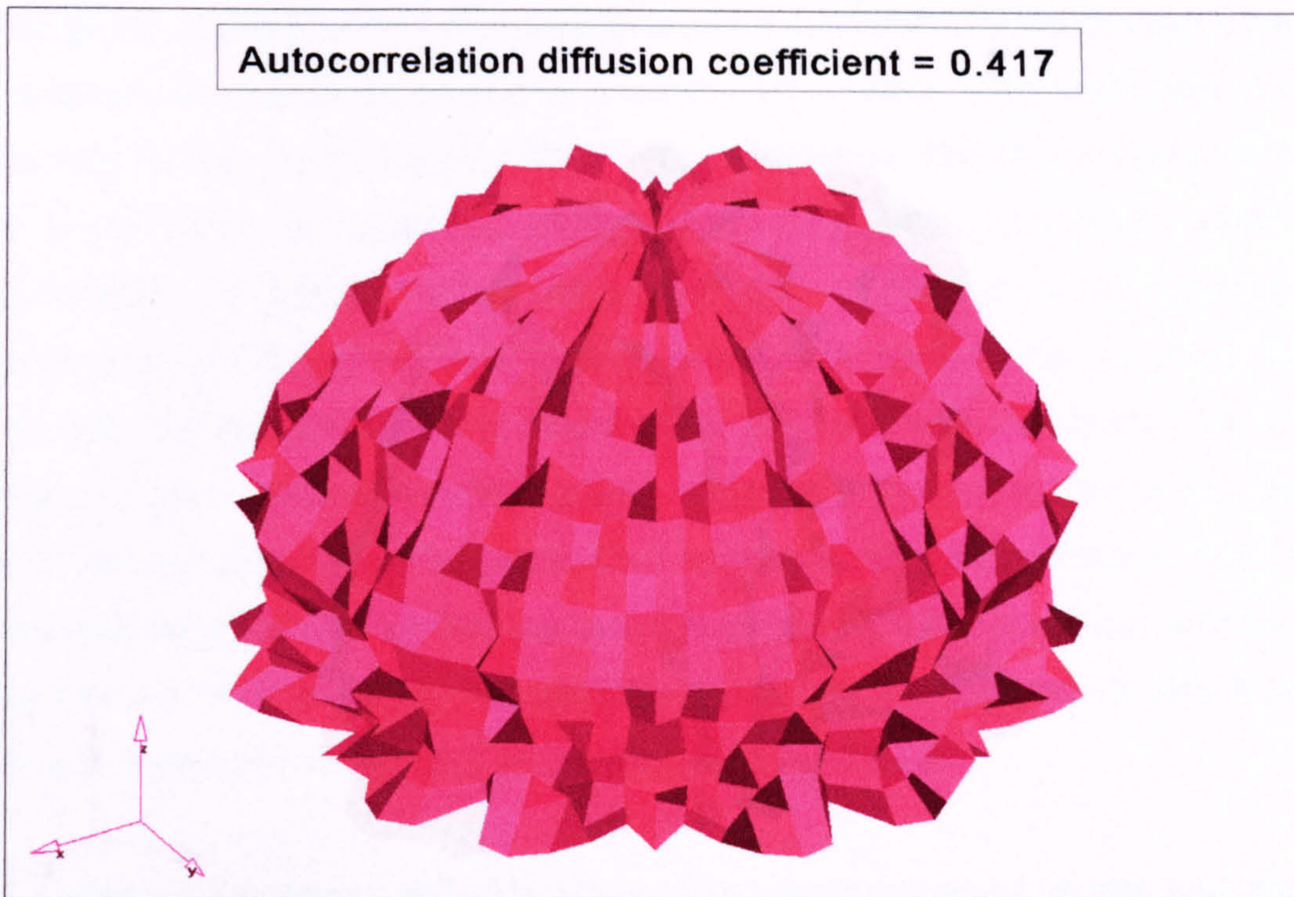
Figure 3.57: 160Hz normal incidence polar response of the plane hexagon, measured at Salford.
