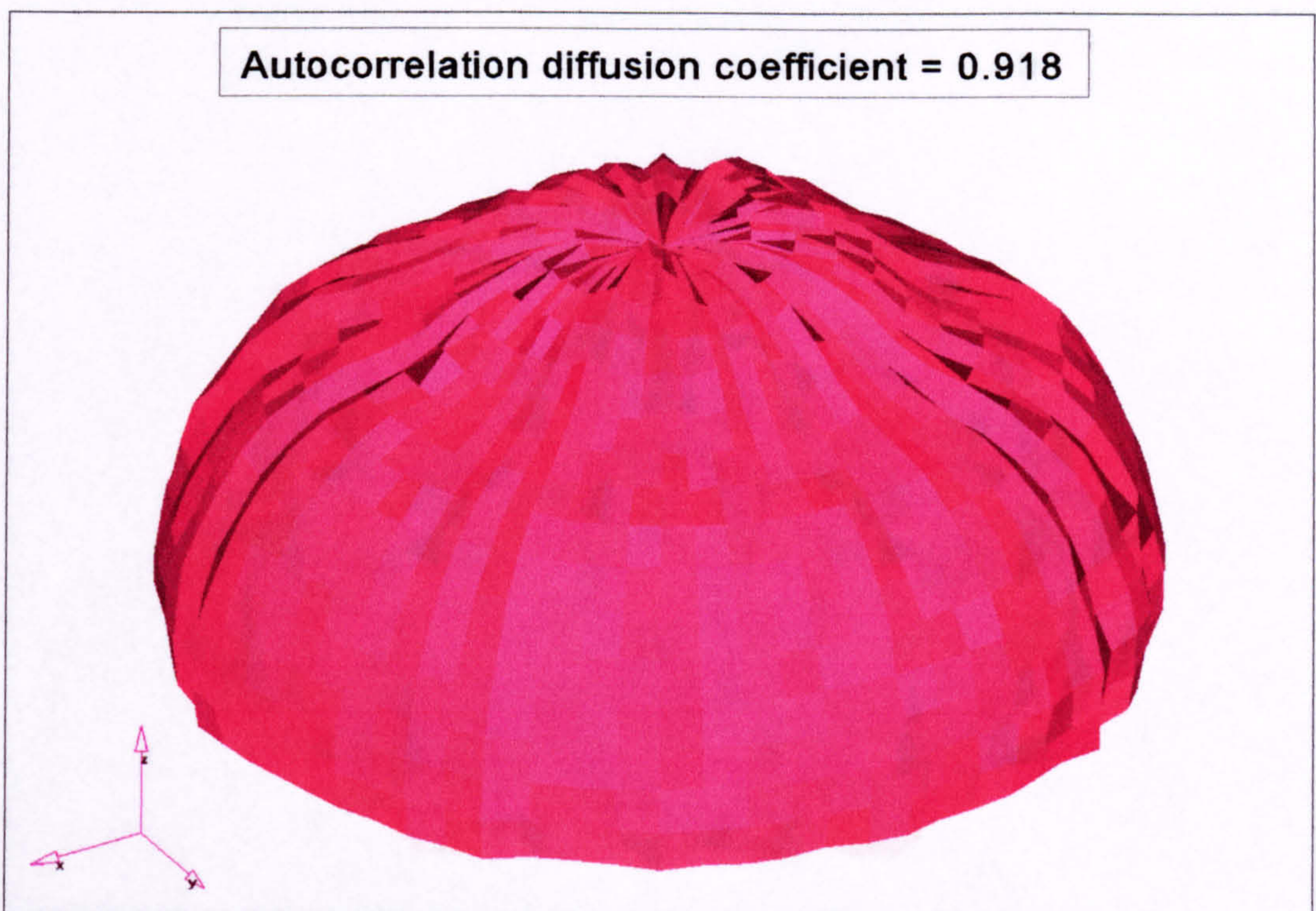
Figure 3.52: 125Hz normal incidence polar response of the Skyline on a 15m (full scale) baffle, measured at Salford. (Essentially the response of the baffle.)
