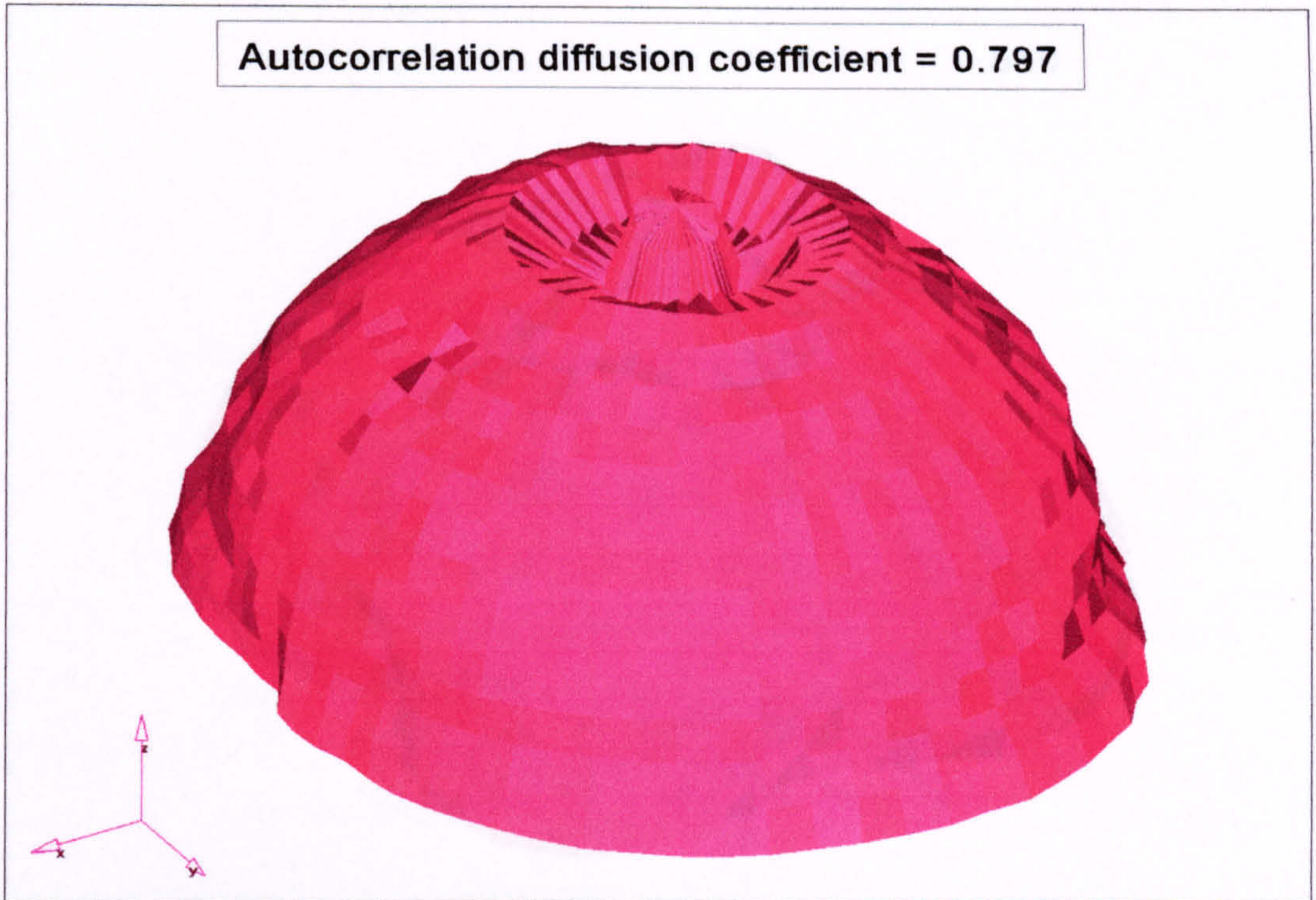
Figure 3.53: 800Hz normal incidence polar response of the Skyline on a 15m (full scale) baffle, measured at Salford. (Essentially the response of the baffle.)
