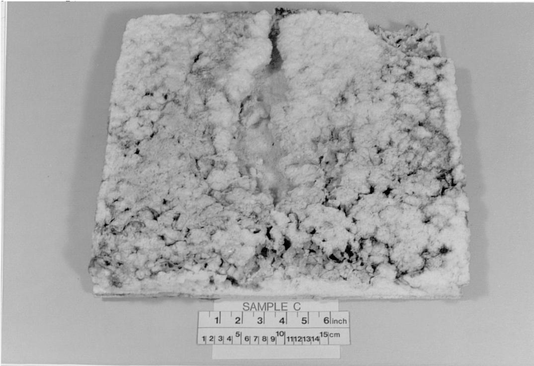
**Plate 9.1 Intumescence Foam Filling the Space Occupied by the Honeycomb core**
