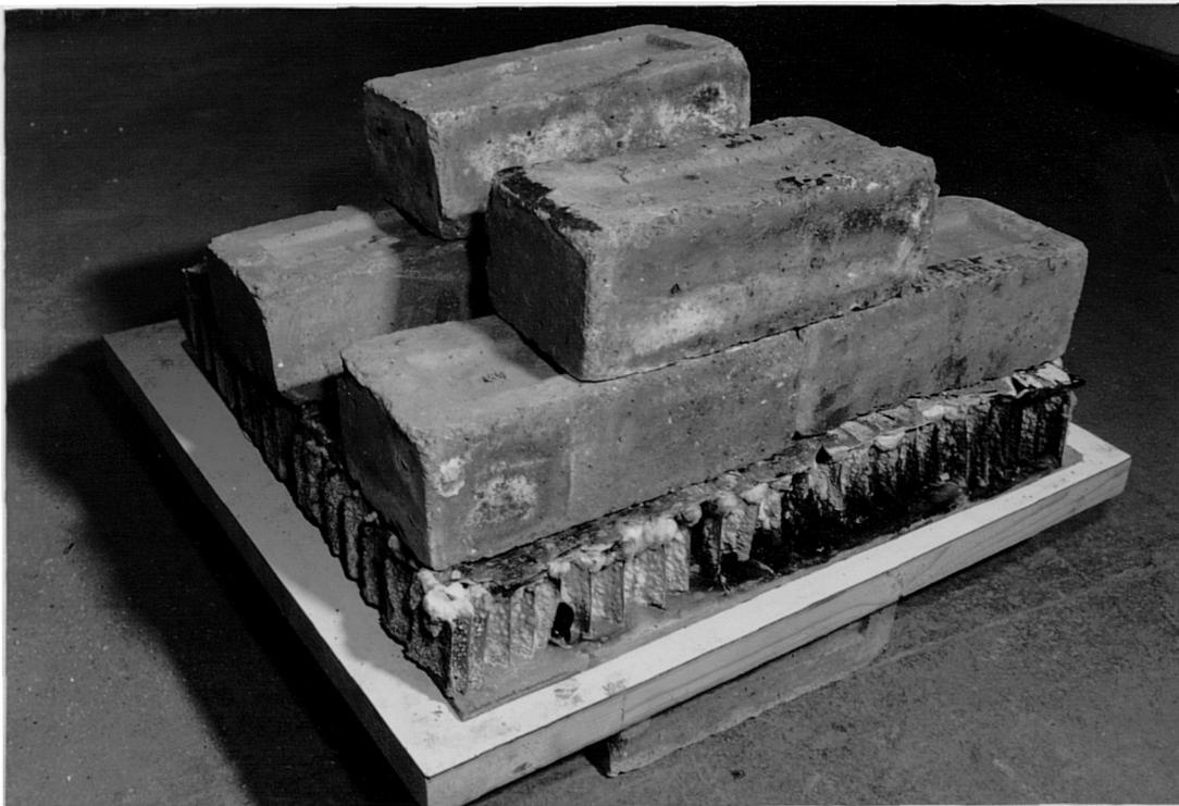
**Plate 9.6 Strength retention at High Temperature of Sodium Silicate and Vermiculite Coating**
