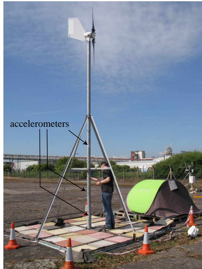
Figure 5 Photograph of a “flat roof” mounting system on test site, also showing some of the accelerometers.
