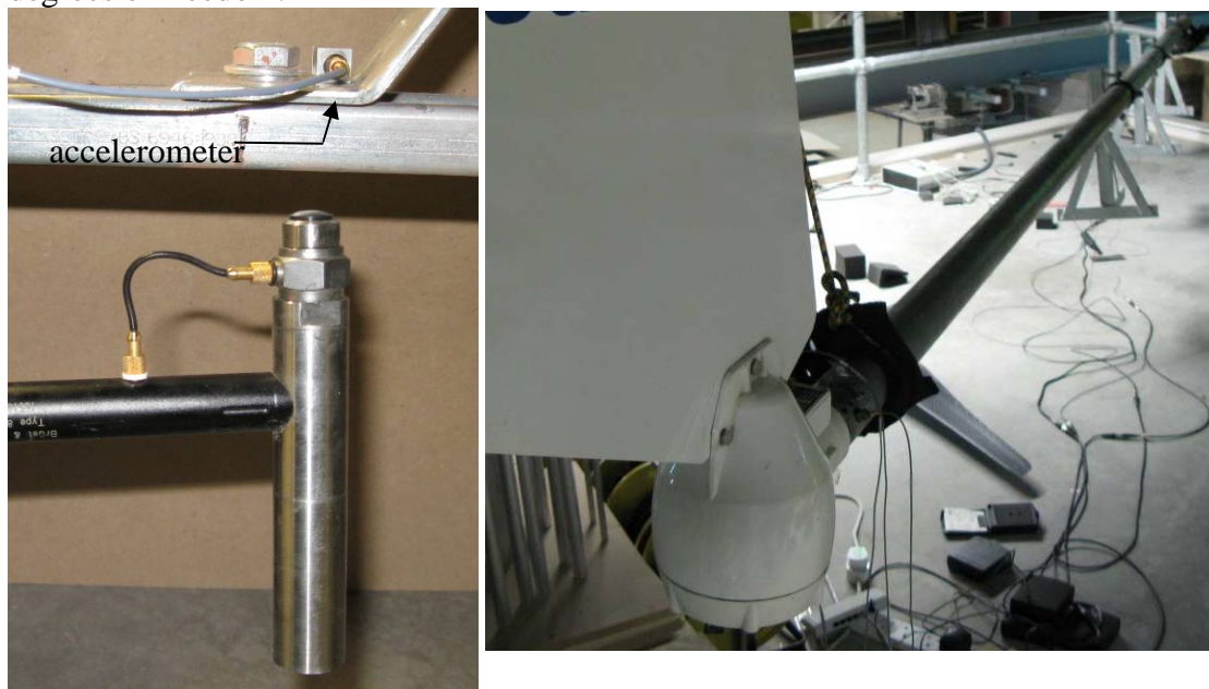
Figure 36: Set up for testing of the mount transmissibilities. Left: force hammer and accelerometer. Right: mast in suspended position for testing.
