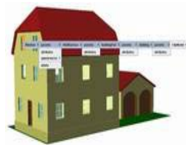
Buildings in LOD 3, automatically generated from IFC building objects.
