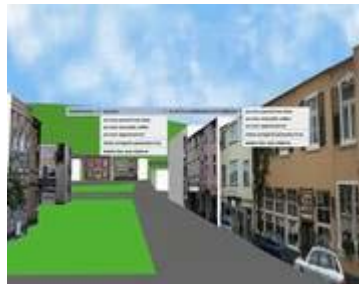
Simple model of the city Königswinter including LOD 1 buildings, terrain, and streets
