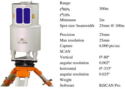
Table 1: Specification of LMS Z210 scanner used in the case study area
