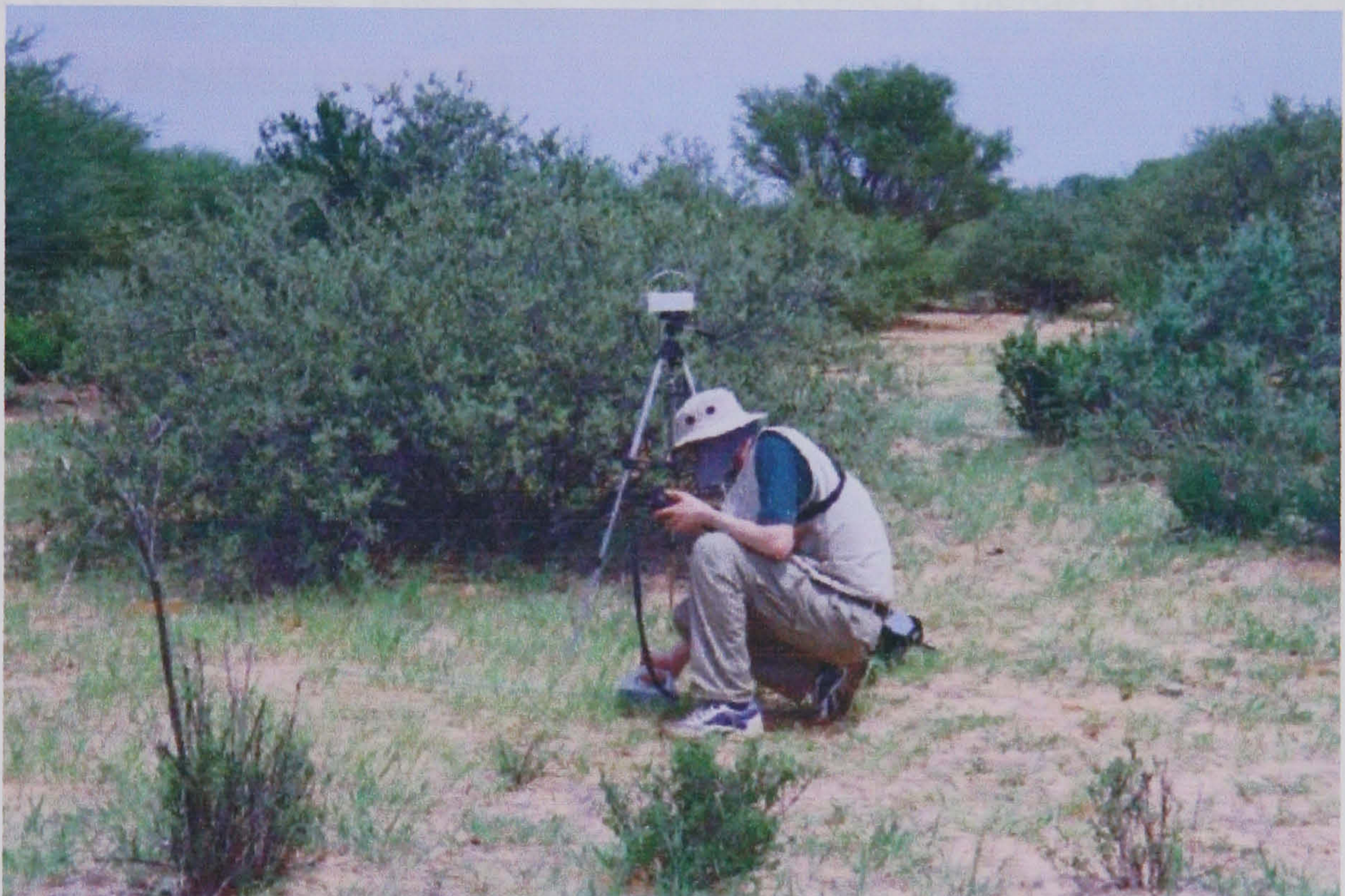
Figure 4.2 Measurements of PAI with the SunScan plant canopy analyser, at Tshane plot 1. Top, overstorey measurement, showing the SunScan probe and; bottom, understorey measurement, showing the SunScan probe, beam fraction sensor (with shadow ring).
