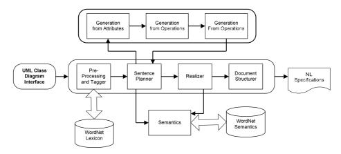
Fig. 1. The GeNLangUML System's Architecture
