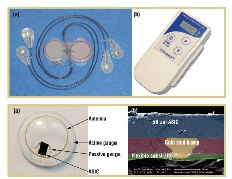
Figure 5. Glaucoma sensor (a) contact lens and (b) ASIC assembly.
