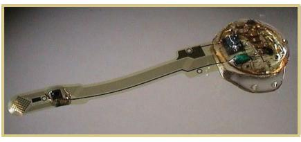
Figure 2. Retinal stimulator for the Healthy Aims retinal implant system. The electrode array is  $4 \times 5.5$  mm, and the electronics is approximate 25 mm in diameter.
