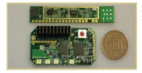
Zarlink has integrated the MICS chip into two FES implants, one for upper arm movement and the other for bladder control. University College London and Finetech Medical are now working to integrate the chip and antenna into the implant enclosure. Figure 8 shows a demonstrator, now available from Zarlink, that includes a processor to prove the communication link. For more details on this project, see *Body Sensor Networks*, chapter 4.
