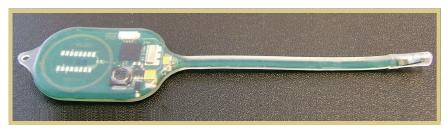
Figure 6. Fully implantable wireless sensor for the intracranial pressure monitoring system.
