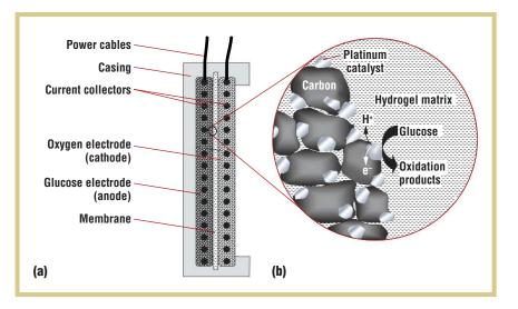
The consortium partners, University of Freiburg (IMTEK) and University of Rovira i Virgili (DINAMIC), characterized the fuel cell's electrochemistry in tests carried out at 37°C in 600 ml of aerated phosphate-buffered saline solution (pH 7.4) containing 0.1 percent glucose by weight (the appoximate concentration of human interstitial fluid). A stable power output of 1.5  $\mu$ W/cm<sup>2</sup> was observed after 200 days, with a corresponding cell voltage of 112 mV.
