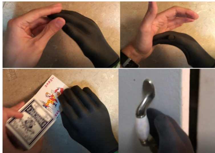
Figure 11. Passive hand being tested for flexibility, friction, and opening a cabinet using the handle.
