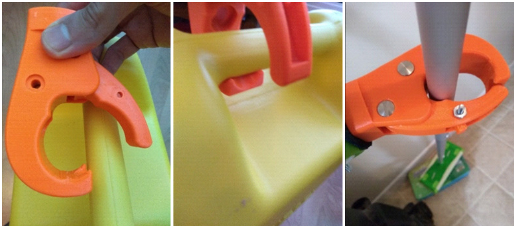
Figure 8. Inner profiles provide the shape to lock around handles for controlled manipulation.
