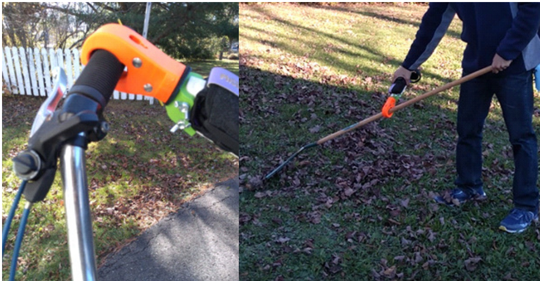
Figure 12. Bicycle handle with rubber grip provides secure hold for prehensor. Long smooth handled garden equipment result in varying degrees of gripping success. A garden rake is easy to manoeuvre because it does not have to carry a heavy load, providing the user with a greater sense of control.
