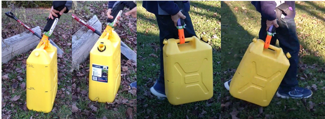
Figure 14. The prehensor is used to lift a load of 12.9 kg. As the arm swings in the first few steps, the prehensor moves to a stable position towards the rear of the handle.
