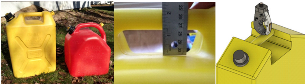
Figure 7. The taller 20 L yellow jerry has a smaller handle opening than the red jerry can and was used to determine dimensions for the inner profile of prehensor.
