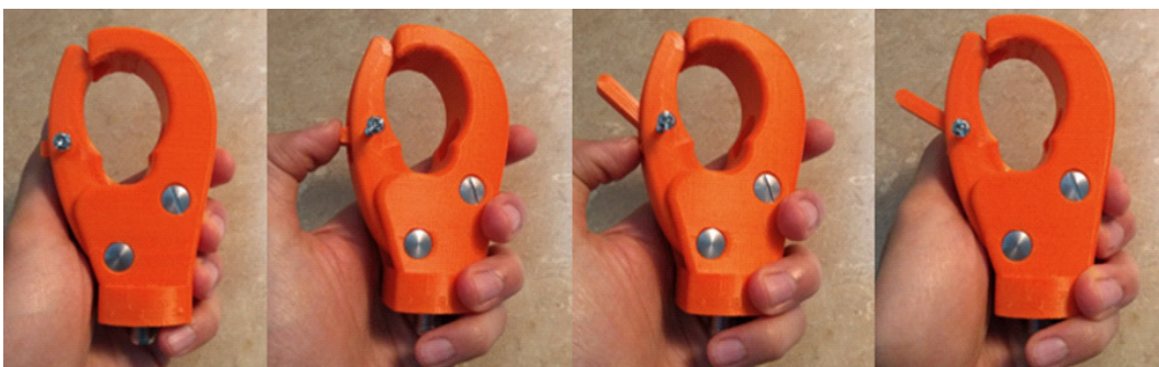
Figure 5. Trigger lever is concealed inside thumb and is rotated outward when needed for opening the terminal device.
