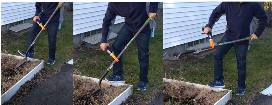
Figure 13. Use of a garden shovel begins with an impact force (foot used to drive shovel into ground), proceeds to a lever action (prehensor is the fulcrum) and then a final lifting force. A lack of secure grip on the handle causes the prehensor to move to different location on the handle which creates uncertainty for the user.
