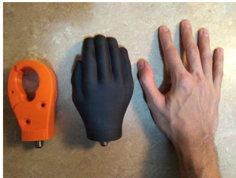
Figure 15. From left to right: prehensor, passive hand, adult male hand.
