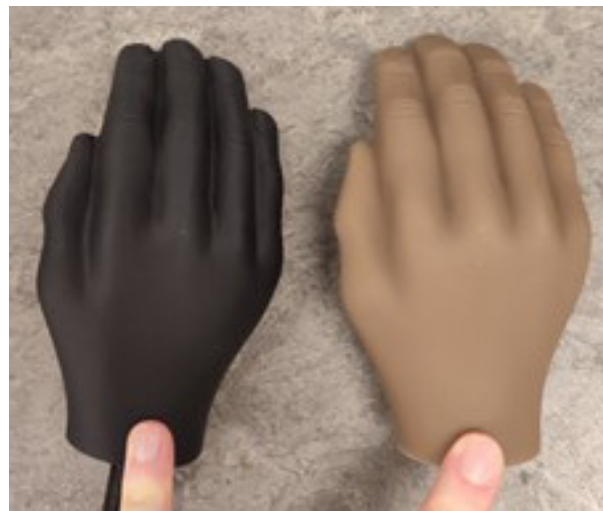
Figure 3. The commercial terminal device (tan colour) and the 3D printed device (black) The passive hand required approximately 40 h to print. This 3D printed hand did not include a ½-20 threaded bolt for mounting to a prosthetic arm but served the purpose of Co-design2.
